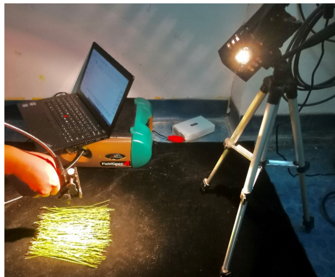
Figure 4. Spectral data acquisition setup.
