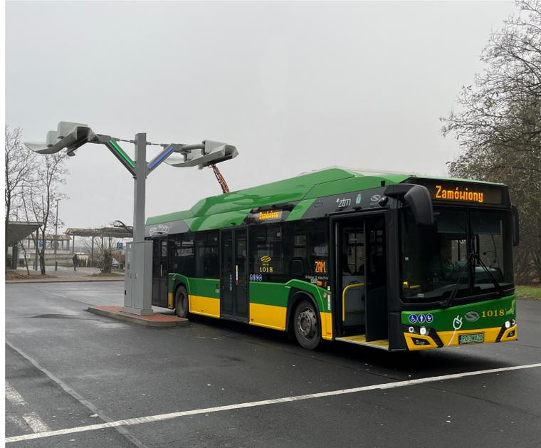
Figure 8. The electric urban bus, Solaris Urbino 12 Electric, used for the experiment in this work.
