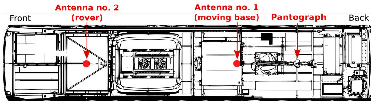
**Figure 2.** Mounting positions of the GNSS antennas with respect to the geometry of a bus roof. The first antenna, connected to the moving base receiver, is mounted 0.2 m ahead of the rear axle and provides the position of a vehicle. The second one, connected to the rover module, is mounted 5 m in front of the first one and is used to calculate the bus heading.
