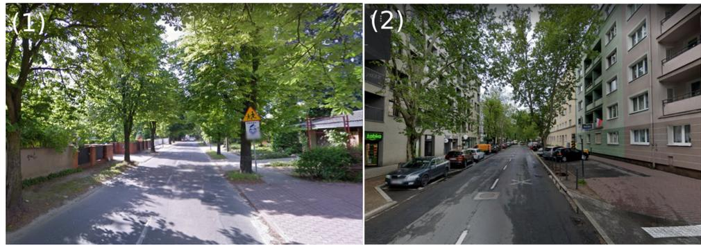
**Figure 5.** Exemplary parts of the trajectories, where the RTK FIXED mode of GNSS was not available because of the poor sky visibility caused by buildings and trees. Image (1) presents the part of the trajectory from Figure 4B, while image (2) shows an example scene from Figure 4C.
