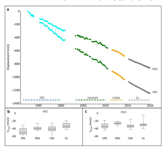
**Figure 7.** (a) Cumulated Vslope displacement time series (1992–2020) spatially averaged of the PS covering the PDR and ARZ hamlets; (b) Box-plot of Vslope distribution for each satellite dataset used on the ARZ hamlet; (c) Box-plot of Vslope distribution for each satellite dataset used on the PDR hamlet.
