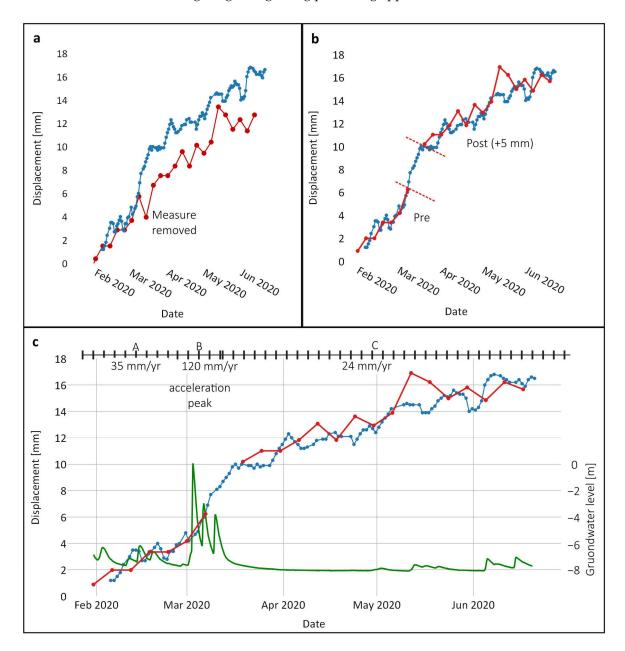
**Figure 10.** Comparison between AIS displacements (top of the borehole) and InSAR data from Sentinel-1 EGMS for February–July 2020 at the PDR site. (a) Original Sentinel-1 EGMS time series showing underestimation; (b) EGMS time series divided into pre- and post-acceleration events, the post-event time series is shifted by +6 mm; (c) AIS and InSAR time series compared with GWL data.
