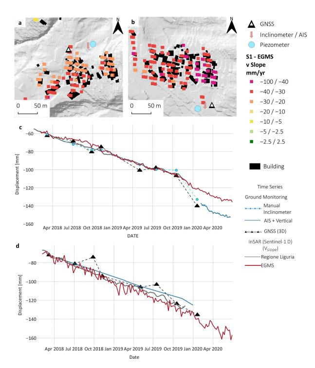
**Figure 11.** Sentinel-1  $V_{slope}$  data and location of ground instruments for PDR (a) and ARZ (b). Comparison of displacement time series of MT-InSAR of Sentinel-1 ( $V_{slope}$  descending dataset), GNSS (3D component) and inclinometers/AIS (with the vertical component from SAR) for the period of overlapping measure (April 2018–June 2020) for the sites PDR (c) and ARZ (d).
