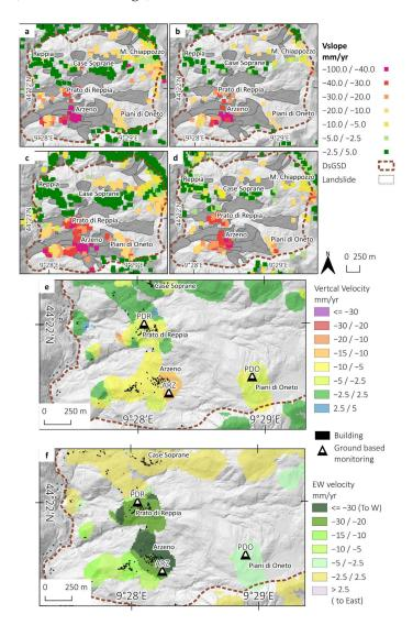
**Figure 6.** InSAR data results over the Arzeno–Prato study area. Shown is the velocity along the line of sight ( $V_{LOS}$ ) for the descending geometry of (**a**) ERS, (**b**) Envisat, (**c**) Cosmo-Skymed, (**d**) Sentinel-1 satellites. With ascending and descending geometries of Sentinel-1, it was possible to resolve the vertical panel (**e**) and East-West panel (**f**) components of the velocity.
