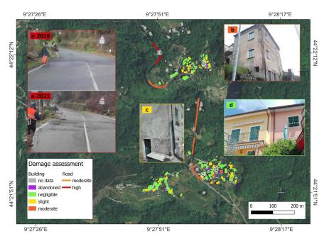
**Figure 3.** Damage assessment in the study area. (a) Road cracks and displacements in 2016 and 2021; (b) moderate damage on an abandoned building in PDR; (c) slight damage on an old building in ARZ; (d) negligible to slight damage in a recent maintained building in ARZ.
