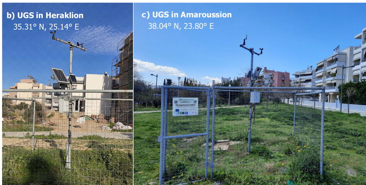
Figure 1. (a) Map of the sites and (b) photos of the meteorological stations installed in the urban green spaces (UGSs) of (a) Heraklion (S. Greece—Crete island), and (c) Amaroussion (central Greece).
