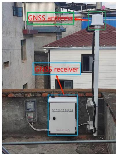
Figure 3. Data acquisition equipment.
