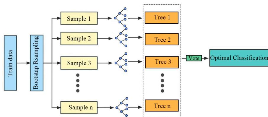
**Figure 4.** Schematic diagram of the RF model.
