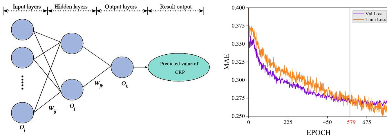
**Figure 5.** Schematic diagram of the MLP model. O represents the neuron, W represents the weight, and the broken line represents the variation in MAE with the number of iterations (EPOCH). 579: we return the model weights for the 579th iteration.
