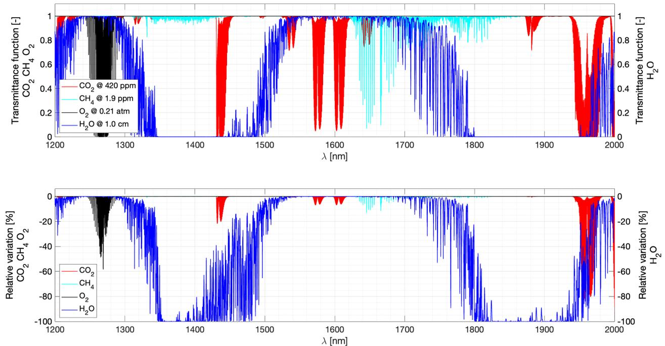
**Figure 4.** (top) Dimensionless transmittance functions ( $TR(\nu, T, P, L)$ ) for CO<sub>2</sub>, CH<sub>4</sub>, O<sub>2</sub>, and H<sub>2</sub>O as a function of wavelength and for nominal mixing. (bottom) Dimensionless transmittance functions' relative variations from a 'maximum' mixing ratio (430 ppm for CO<sub>2</sub>, 2.0 ppm for CH<sub>4</sub>, 0.22 for O<sub>2</sub>, and 1.1 precipitable cm for H<sub>2</sub>O) to a nominal mixing ratio.
