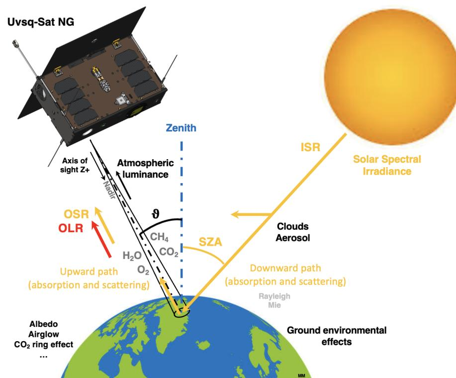
**Figure 3.** Schematic illustration of radiation transfer in passive remote sensing, applied to Uvsq-Sat NG. The observation approach of the Uvsq-Sat NG NIR Spectrometer relies on measuring spectra of sunlight scattered back via the Earth's surface and atmosphere in the NIR spectral range.
