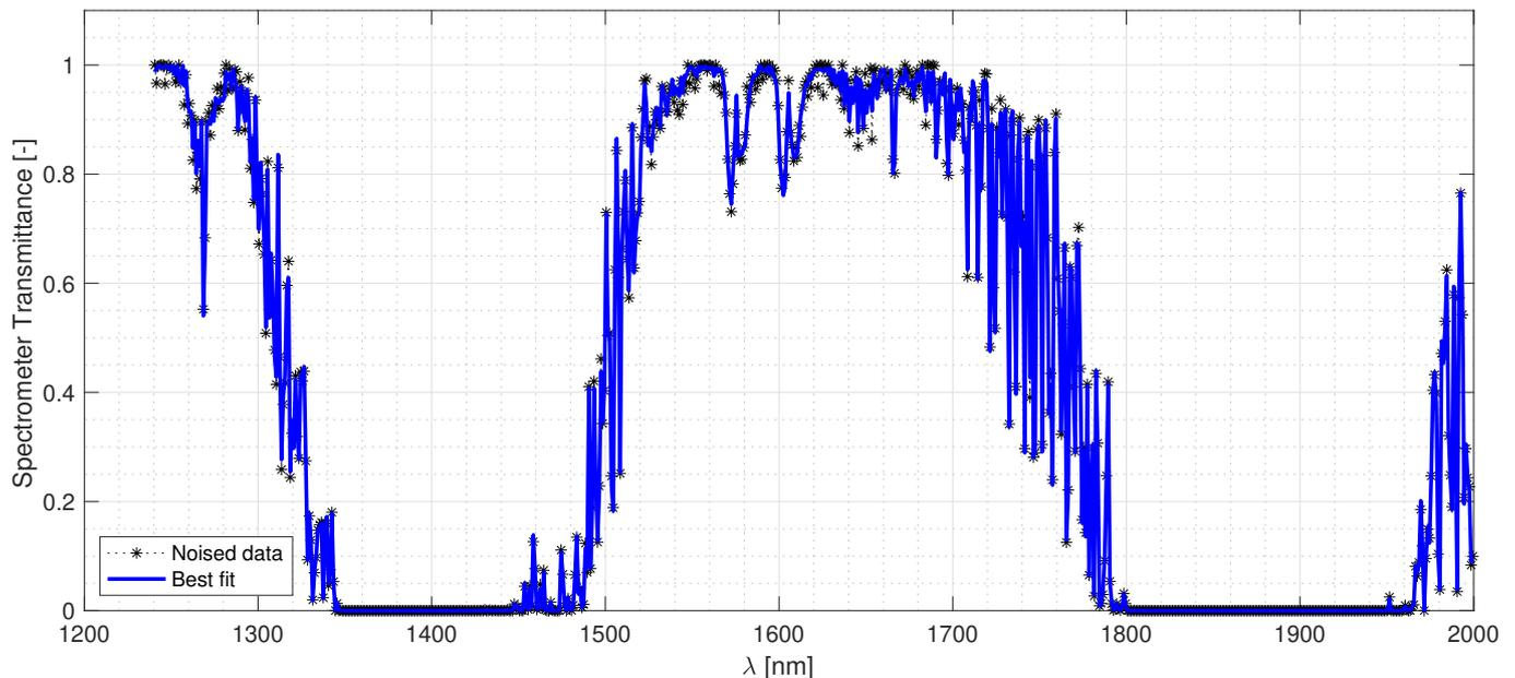
**Figure 6.** Uvsq-Sat NG NIR Spectrometer data retrieval of the dimensionless signal ( $TR_{Spectro}(\lambda)$ ) as it can be observed via the spectrometer (spectral resolution of 1 nm and SNR of 50). The dark stars (noised data) represent data of the dimensionless signal (Step 4). The blue curve represents the best fit obtained using the Levenberg–Marquardt algorithm (Step 5).
