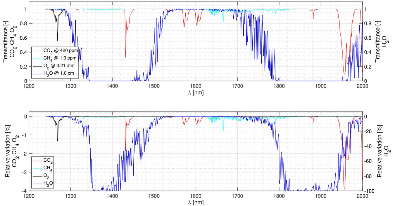
**Figure 5. (top)** Dimensionless transmittance functions at the Uvsq-Sat NG Spectrometer resolution assuming a spectral resolution of 1 nm (FWHM) for the spectrometer. A Gaussian convolution filter is used. **(bottom)** Relative variation between 'maximum' mixing ratio and nominal mixing ratio.
