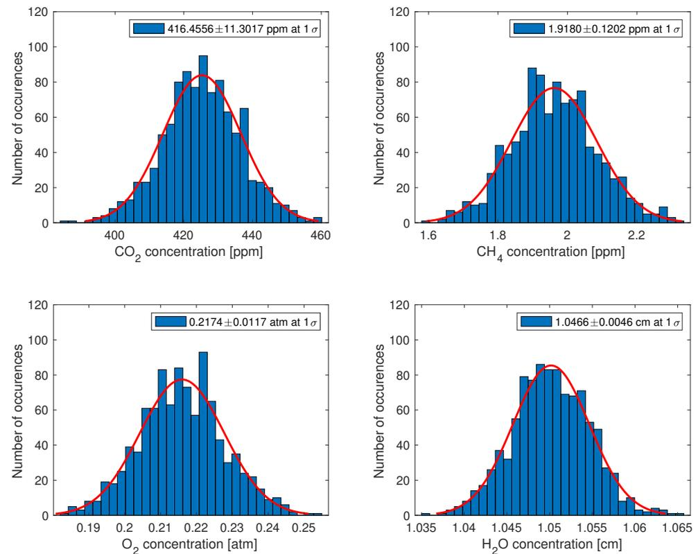
**Figure 7.** Restitution of the concentration of gases observed via the Uvsq-Sat NG NIR Spectrometer. In this simulation, the spectrometer has a resolution of 1 nm and a SNR of 50.
