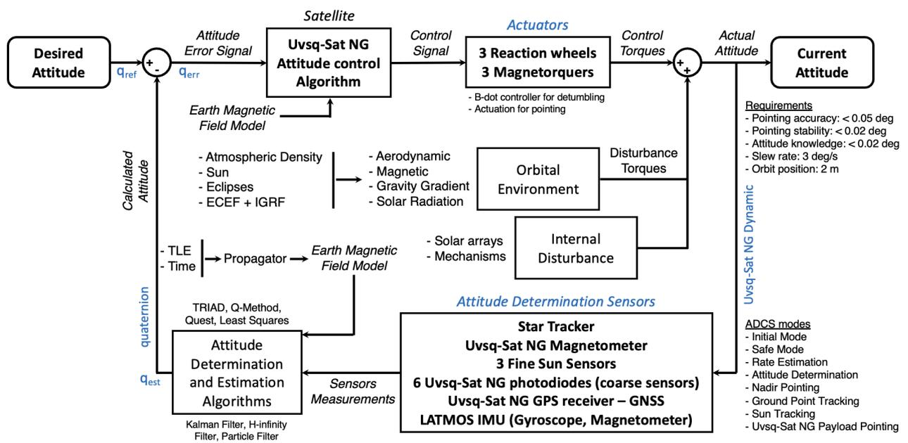
**Figure 2.** General ADCS control loop of the Uvsq-Sat NG CubeSat. Earth-Centered Earth-Fixed (ECEF) is a coordinate system that defines positions in relation to the Earth’s center while considering the Earth’s rotation. It provides a fixed reference frame for navigation and positioning calculations.
