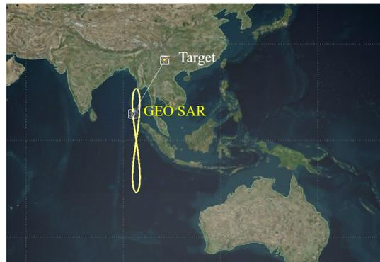
**Figure 6.** Trajectory diagram for GEO SAR based on the orbital elements.
