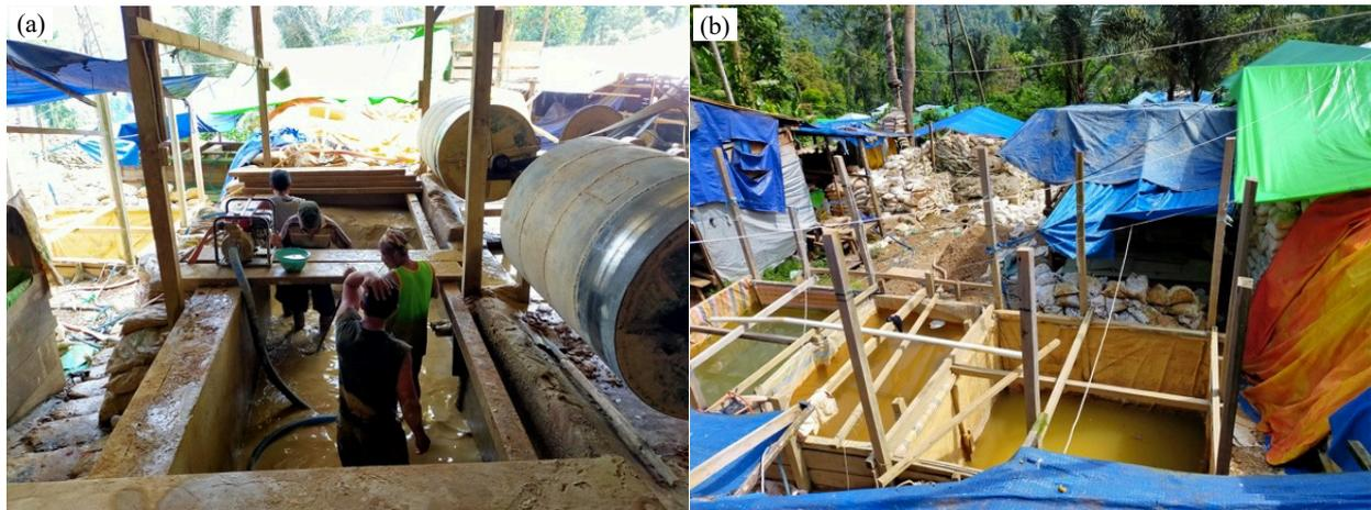
**Figure 3.** Pools of water mixed with hydrogen peroxide (a) and mercury mixed with cyanide (b) for immersing materials in the study sites [22].
