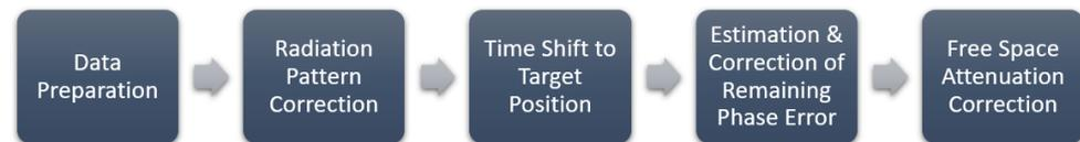
**Figure 5.** Signal processing steps for a single measurement setup.
