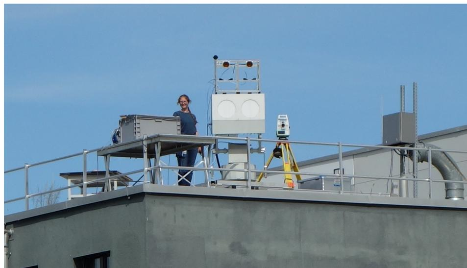
**Figure 2.** Photo of the elevated measurement set up located on the top of a building. The VNA is placed in a temperature-controlled box on the left on a table with its antennas (orange radoms) on top of the transponder (white and gray box on a positioner unit). The geodetic total station is placed on a wooden tripod right of the transponder.
