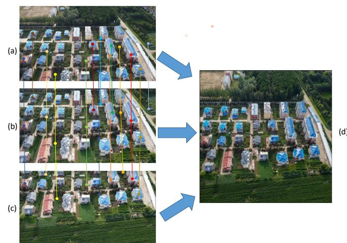
**Figure 8.** The illustration of image mosaic for UAV remote sensing panorama by the proposed video synchronization method. Some detected salient positions among views are displayed and matched by lines. (a–c) display three image sequences with minor time offsets, (d) shows the image stitching result.
