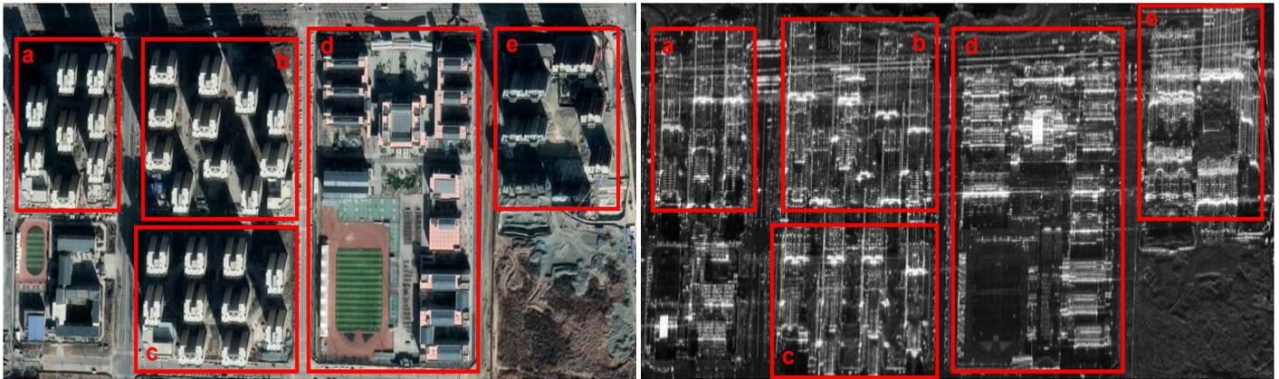
**Figure 7.** Experimental area optical images and corresponding SAR 2D images. The left image is an optical image, while the right image shows the corresponding SAR 2D images. The red boxes labeled from “a” to “e” indicate the five selected regions in the experiment.
