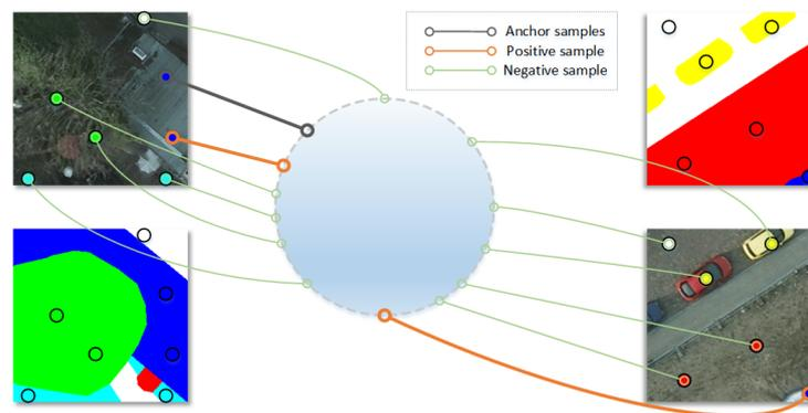
**Figure 2.** Scheme of supervised contrastive learning module for semantic segmentation.
