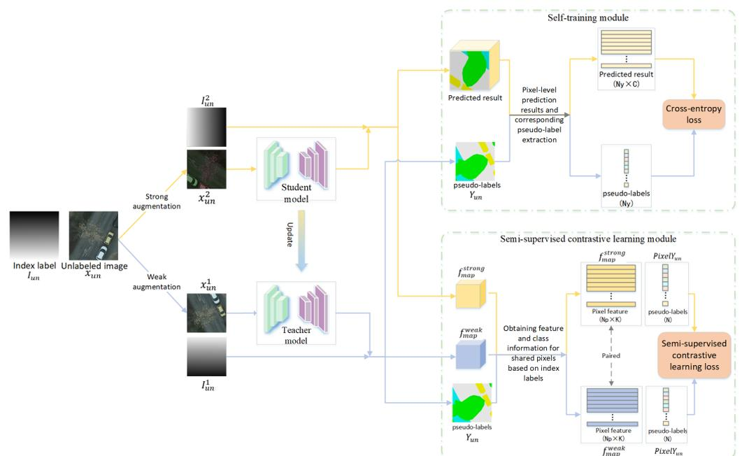
Figure 3. The self-training module and semi-supervised contrastive learning module.
