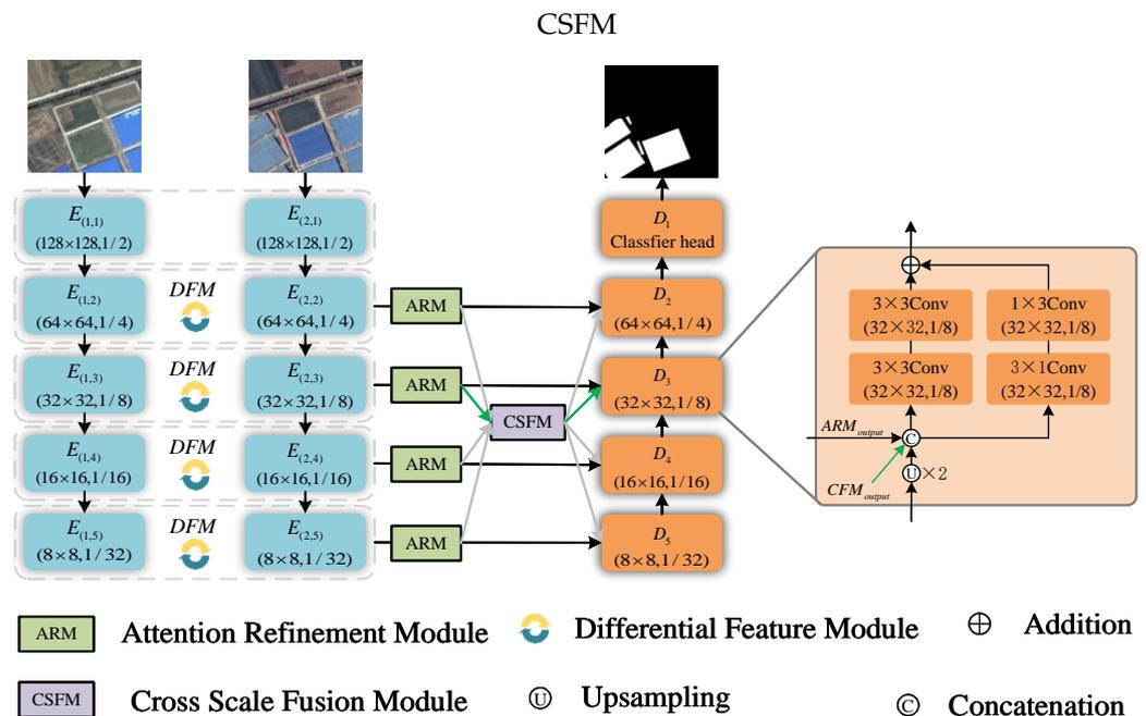
**Figure 1.** The overall framework of MDANet. Incorporating ResNet34 as the primary backbone network for decoding, the network has an encoder–decoder architecture.
