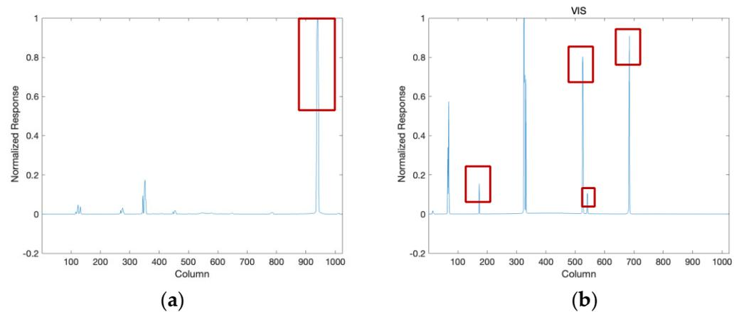
**Figure 16.** OMS-N response to the standard spectral lamp, and the red rectangle shows the selected standard spectral line. (a) UV band; (b) VIS band.
