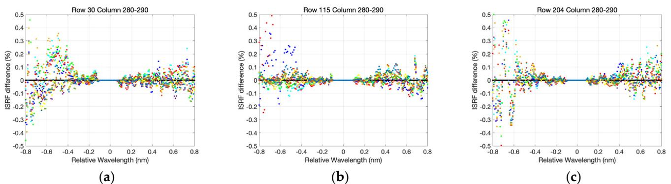
**Figure 7.** The ISRF difference in the VIS band between the center (column 285) and the others (columns 280–290). The different dots donate the ISRF differences in different columns. (a) Row 30; (b) row 115; (c) row 204.
