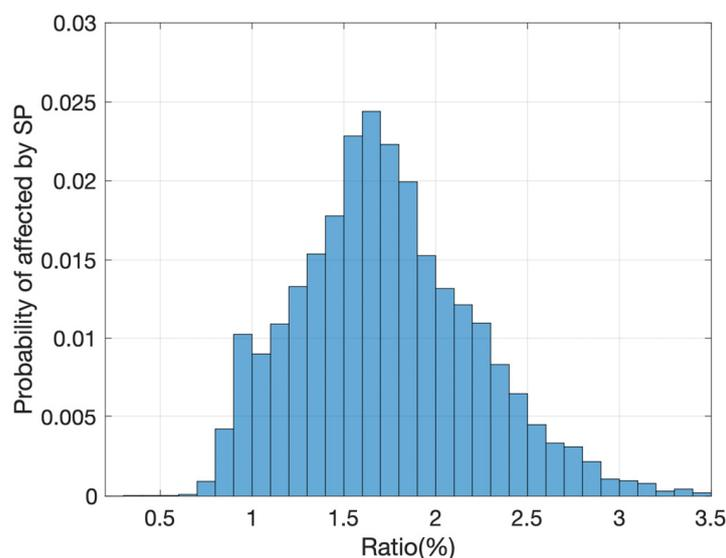
**Figure 17.** Histogram of the response ratio distribution of the ISRF “secondary peak” for all affected pixels in the UV1 band.
