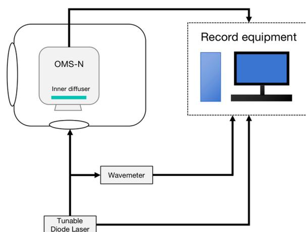
**Figure 2.** Schematic diagram of OMS-N spectral calibration.
