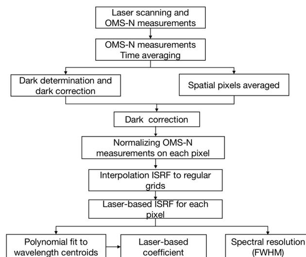
**Figure 3.** Flowchart of the data processing procedure of OMS-N spectral calibration.
