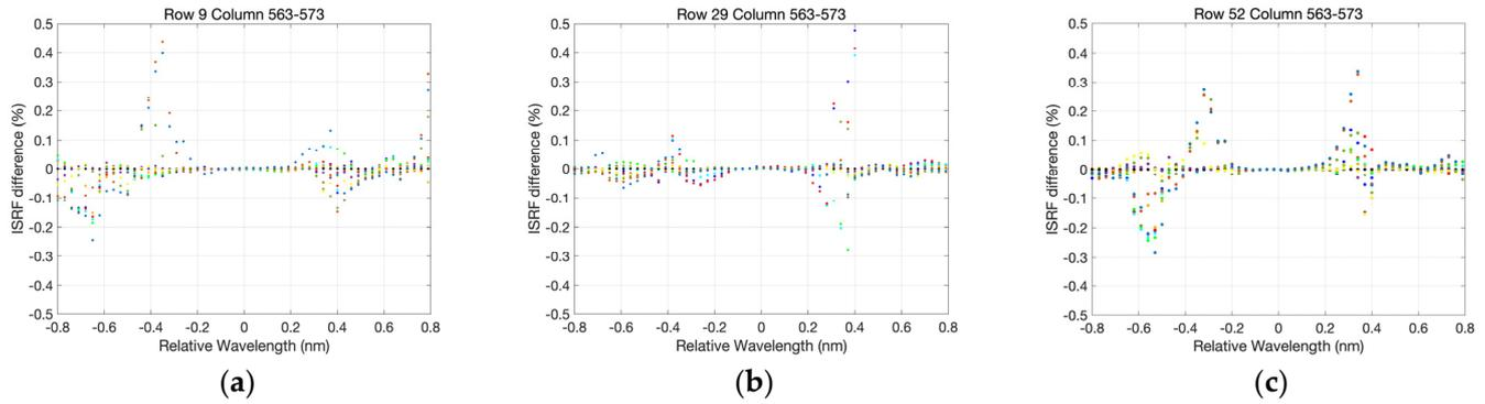
**Figure 8.** The ISRF difference in the UV1 band between the center (column 568) and the others (columns 563–573). The different dots donate the ISRF differences in different columns. (a) Row 9; (b) row 29; (c) row 52.
