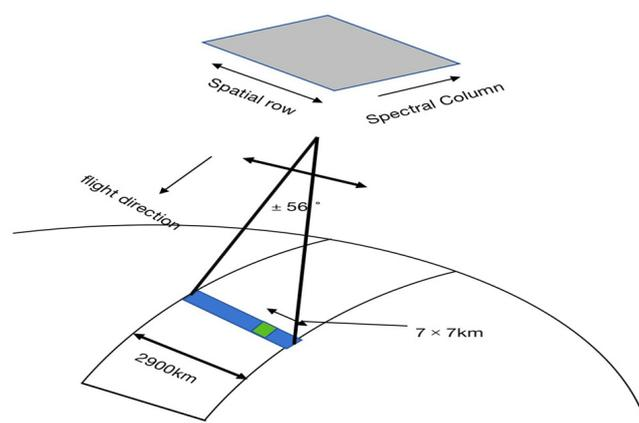
**Figure 1.** Observation schematic view of the FY-3F OMS-N instrument.
