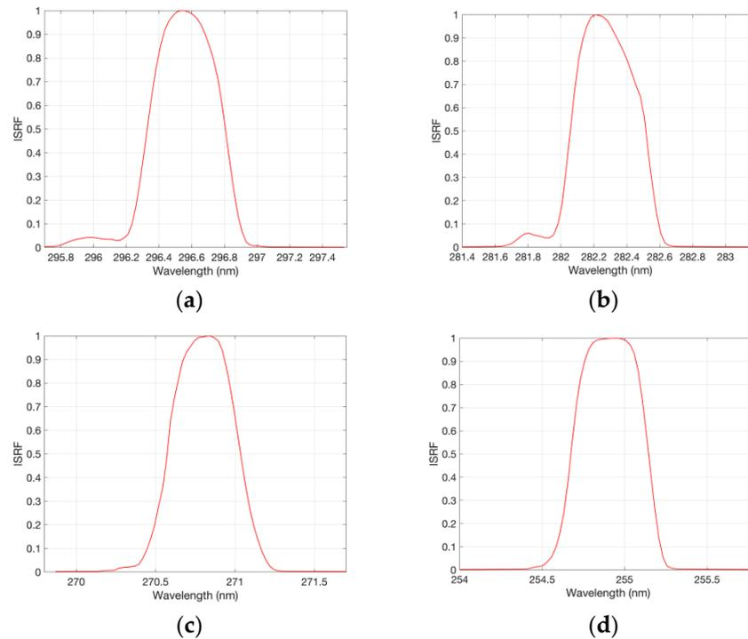
**Figure 6.** The “asymmetric central peak” and “secondary peak” characterization of the ISRF for the nadir row in the UV1 band. (a) Wavelength centroid around 296.6 nm; (b) wavelength centroid around 282.3 nm; (c) wavelength centroid around 270.8 nm; (d) wavelength centroid around 254.9 nm.
