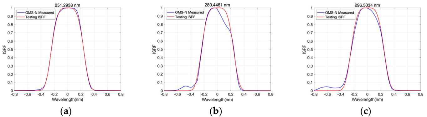
**Figure 18.** An example of the measured ISRF (blue lines) and the testing ISRF (red lines) in the UV1 band. (a) Short wavelength; (b) middle wavelength; (c) long wavelength.
