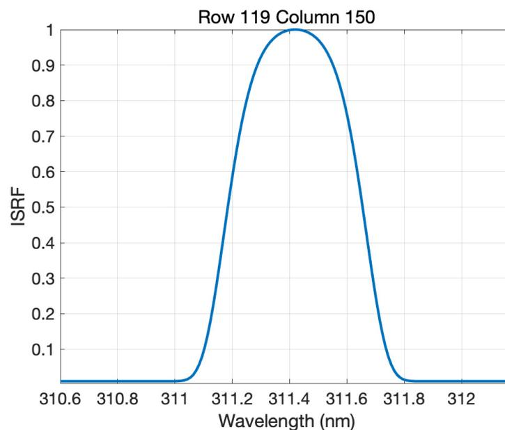
**Figure 13.** The ISRF in the UV2 band for row 119, column 150.
