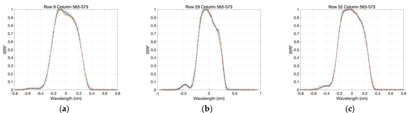
**Figure 11.** Samples from 11 spectral pixels in the UV1 band are combined to give a single set of data, with a higher resolution shown by the colored circles. (a) Row 9; (b) row 29; (c) row 52.
