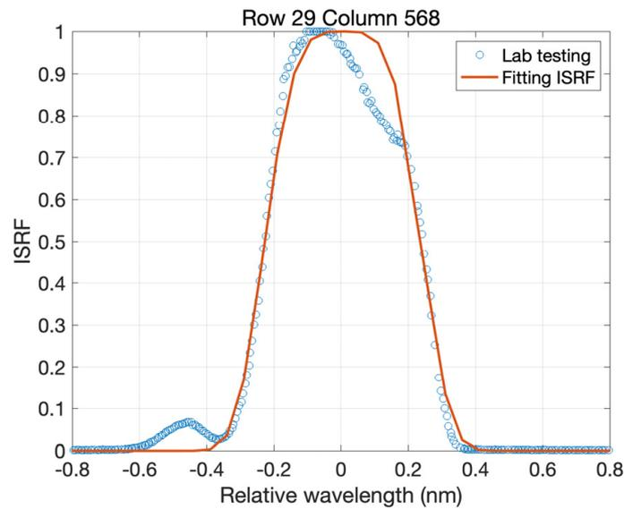
**Figure 12.** Combined ISRF spectral sample data (blue circle) and the fitted ISRF (red line) at row 29, column 568 in the UV1 band.
