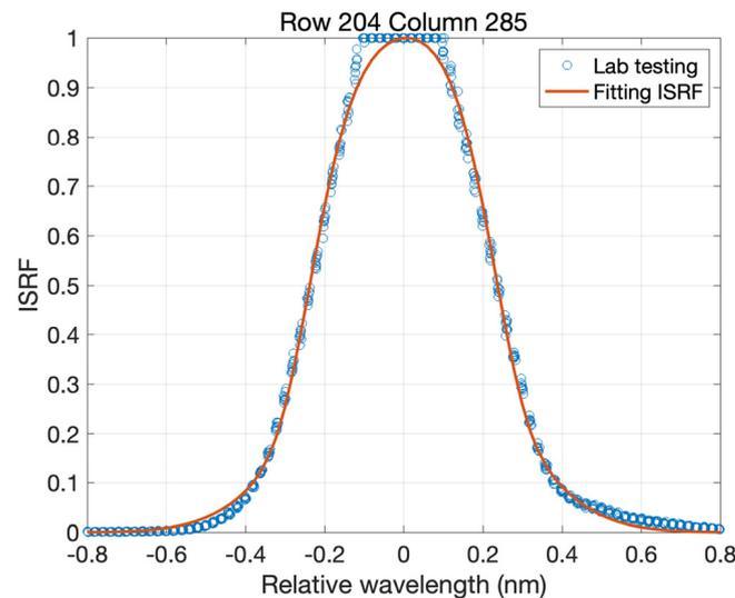
**Figure 10.** Combined ISRF spectral sample data (blue circle) and the fitted ISRF (red line) at row 204, column 285 in the VIS band.
