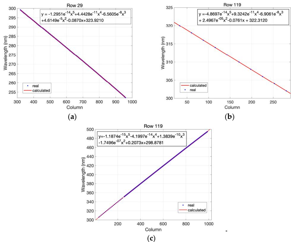
**Figure 15.** Fifth-order polynomial fits (red line) for nadir row wavelength centroids derived from (blue dots) laser data as a function of the spectral pixel index. (a) UV1 band; (b) UV2 band; (c) VIS band.
