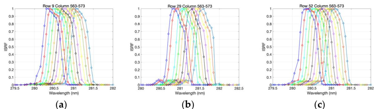
**Figure 5.** Response from a set of 11 spectral pixels (different colors) in the UV1 band. (a) Row 9; (b) row 29 (the nadir row); (c) row 52.
