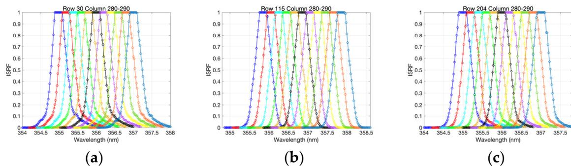
**Figure 4.** Response from a set of 11 spectral pixels (different colors) in the VIS band. (a) Row 30; (b) row 115; (c) row 204.
