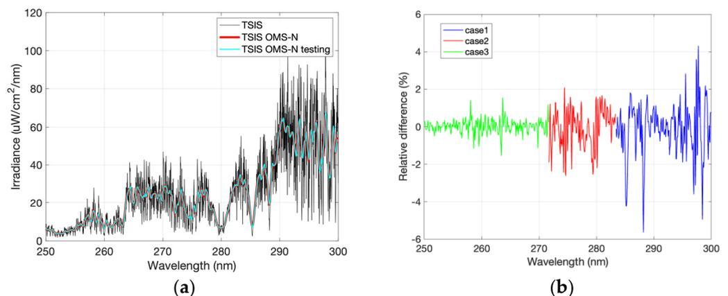
**Figure 19.** The simulated irradiance spectra from OMS-N measured the ISRF (red line) and the testing ISRF (light blue line) and their relative irradiance difference. (a) Simulated irradiance spectra; (b) relative irradiance difference between simulation from the measured ISRF and the testing ISRF.
