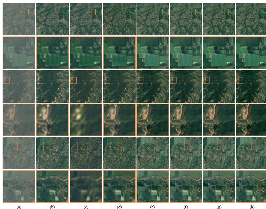
Figure 3. Visualization results of different methods on the RICE1 dataset. (a) Cloudy images; (b) results of the SpA GAN; (c) results of the AMGAN; (d) results of the CVAE; (e) results of the Restormer; (f) results of the TCME; (g) results of ours; (h) ground truth. The enlarged area is indicated by an orange box, and the enlarged result is shown below the original image.
