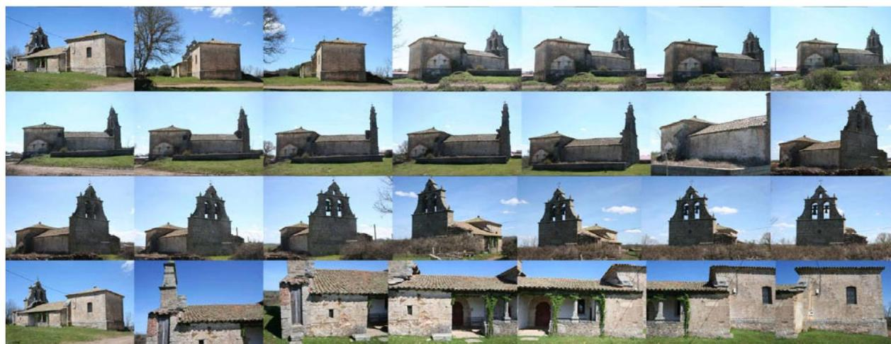
Every church had external conditioning factors (e.g., narrow perimeter streets, fences, private properties, *etc.*), which made it impossible to fit the whole object into the image, at least for one of the façades. In such cases, a planar or mosaic shot of the area was performed, making sure that the images had an overlap rate of at least 80%. We made sure of having convergent (oblique) images to “tie” the circular shots and the mosaic shots in order to obtain a precise orientation.
