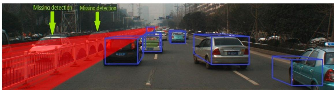
**Figure 8.** Blocked vehicles detection method (guardrail region broadening method). Two vehicles running in opposite directions are missed detection by the vehicle classifier, which are indicated by the yellow arrows. These missed detection vehicle regions are included in the broadened guardrail regions, which are shown as the red region.
