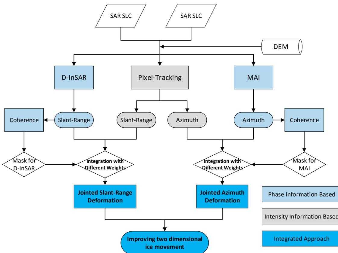
Figure 2. The data processing flowchart of the integrated method.
