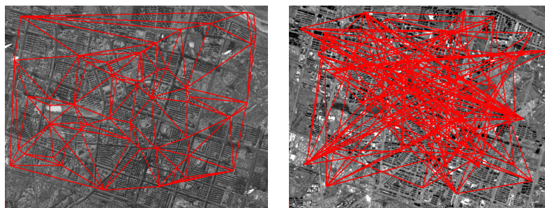
Figure 15. The initial corresponding triangulations produced by TAACC. The false triangle constraints cause mismatches as shown in Figure 14a.
