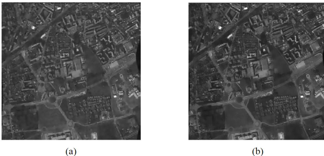
**Figure 2.** Edge preservation of guided filter: (a) Initial de-noised image; (b) Final de-noised image by guided filter.
