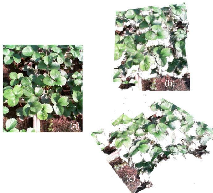
**Figure 16.** The stereo-rectified left image and reconstructed 3D point cloud of greenhouse strawberry samples. The left side (a) is the rectified left webcam image used for generating the 3D point cloud; (b,c) show the reconstructed 3D point cloud of the strawberry sample plants viewed from two different positions.
