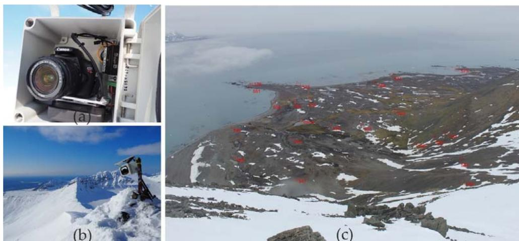
**Figure 2.** Time-lapse camera set: (a) Internal view; (b) Placement near the Fugleberget summit; (c) View from the camera (16 June 2016) with marked location of all the Ground Control Points (GCP) used in the orthorectification process.
