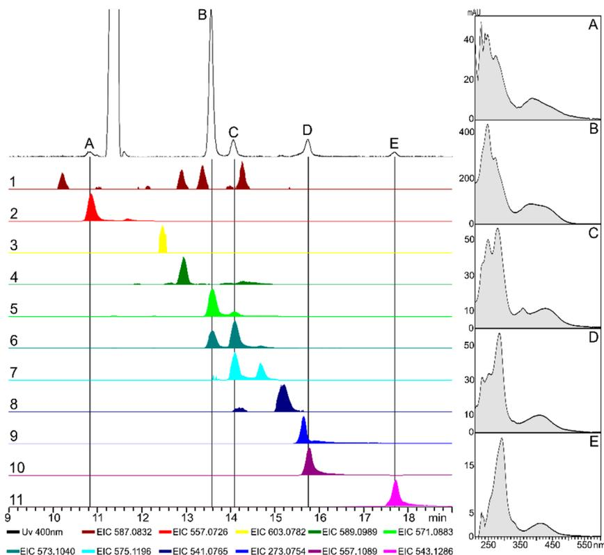
**Figure 4.** Chromatograms from a metabolite extract of Cz medium 5 days after inoculation with OE::*aurR1*. Left: a UV 400 nm chromatogram (spectral background subtracted) with selected peaks (A–E) and underlying colored extracted ion chromatograms (EICs) of selected masses (1–11,  $[M + H]^+ \pm 0.02$  Da) scaled by relative intensities. Right: UV spectra (205–600 nm) for peaks A–E.
