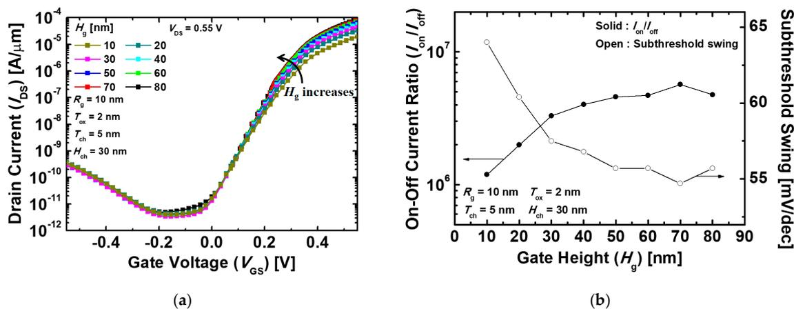
**Figure 5.** (a)  $I_{DS}$ - $V_{GS}$  transfer characteristics and (b)  $I_{on}/I_{off}$  (on-state current/off-state current) and SS of the proposed Ge-based gate-metal-core VNWTFETs with different gate-metal heights ( $H_g$ ).
