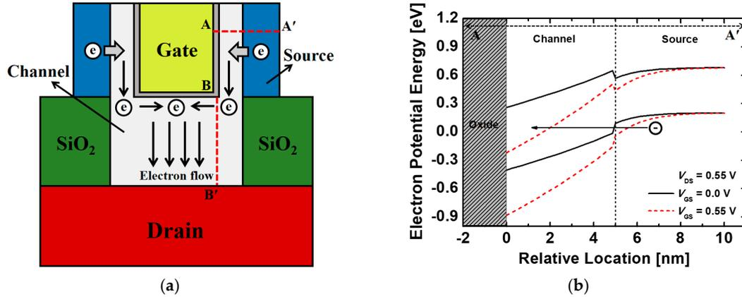
**Figure 2.** (a) The electron flow and (b) energy band diagrams of the proposed Ge-based gate-metal-core VNWFETs. Energy band diagrams are extracted across the A–A’ line in Figure 2a.
