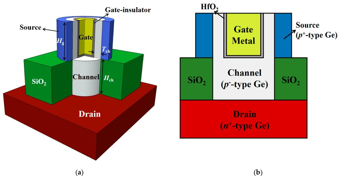
**Figure 1.** (a) Schematic view and (b) cross-sectional view of the proposed Ge-based gate-metal-core vertical nanowire tunnel field effect transistor (VNWTFET), respectively.
