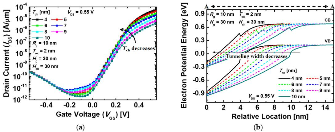
Figure 3. (a)  $I_{DS}-V_{GS}$  (drain current–gate voltage) transfer characteristics and (b) energy band diagrams of the proposed devices with different channel thicknesses ( $T_{ch}$ ). The energy band diagrams are extracted across the A–A’ line in Figure 2a.
