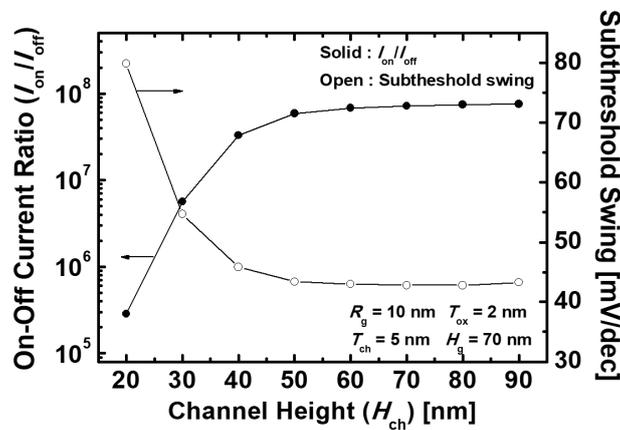
**Figure 7.**  $I_{on}$  and SS characteristics of the proposed Ge-based gate-metal-core VNWTFETs with different  $H_{ch}$ .
