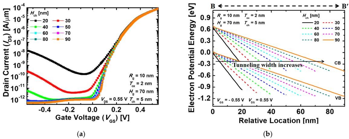
**Figure 6.** (a)  $I_{DS}$ – $V_{GS}$  transfer characteristics and (b) energy band diagrams of the proposed Ge-based gate-metal-core VNWTFETs with different channel heights ( $H_{ch}$ ). The energy band diagrams are extracted across the B–B’ line in Figure 2a at  $V_{GS} = -0.55$  V and  $V_{DS} = 0.55$  V (drain voltage).
