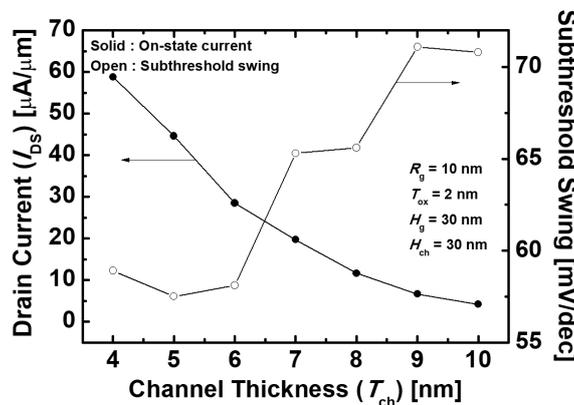
Figure 4.  $I_{on}$  and subthreshold swing (SS) characteristics of the proposed Ge-based gate-metal-core VNWFETs with different  $T_{ch}$ .
