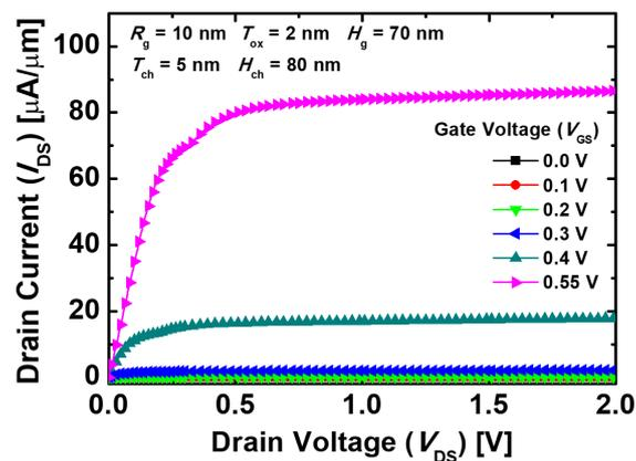
**Figure 8.** Output characteristics of the proposed Ge-based gate-metal-core VNWTFETs with different  $V_{GS}$ .
