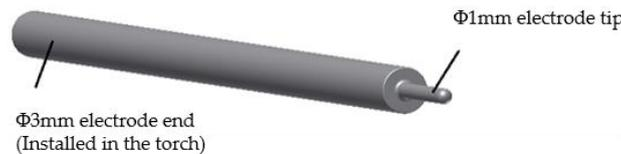
Figure 3. Schematic of needle electrode.
