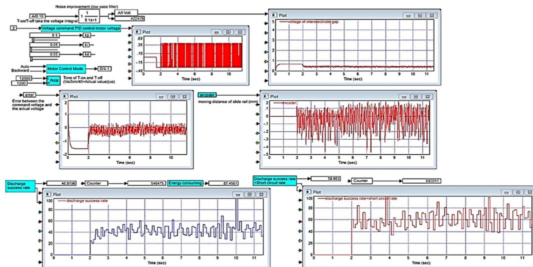
Figure 7. Kp = 0.5, Ki = 0.05, and Kd = 0.05. After Kd increases, error decreases, the discharge success rate increases and the system trends stabilize.
