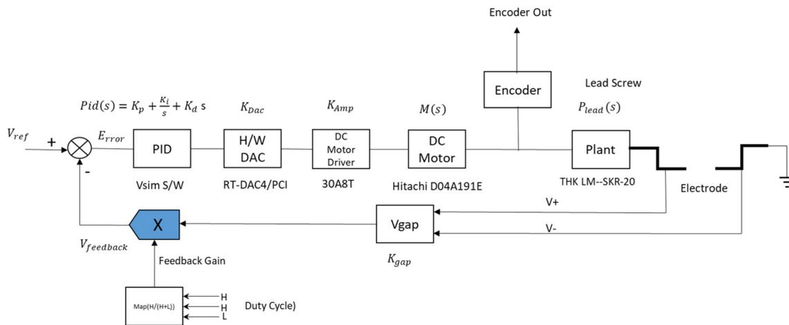
Figure 6. Micro-EDM system parameters.
