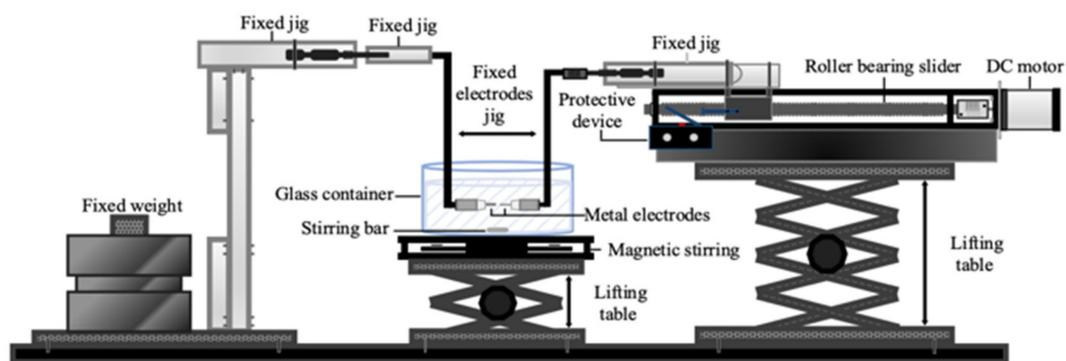
**Figure 2.** Design of micro-EDM.
