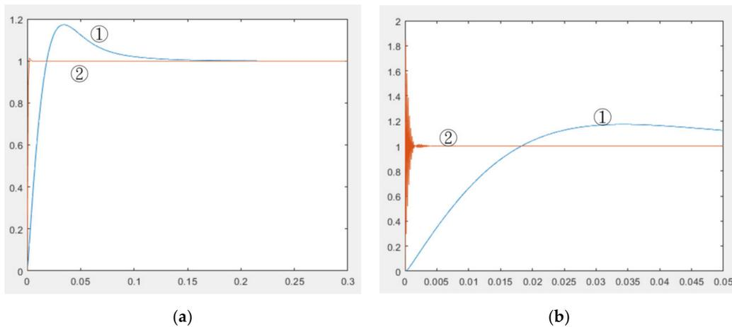
Figure 9. Step response (a) with a sampling time of 1 ms and (b) with a sampling time of 0.1 ms.
