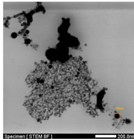
Figure 12. Macroscopic TEM image of bismuth nanoparticles.
