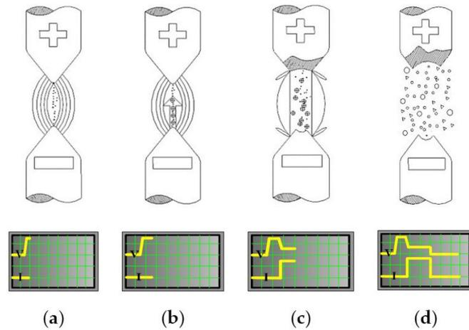
**Figure 1.** Steps involved in nanoparticle formation through micro-electric discharge machine (ESDM). (a) Molecular polarization and formation of a low-resistance channel. (b) Ionization and emission of electrons from the cathode. (c) Metal melt and vaporization. (d) Suspension of particles.
