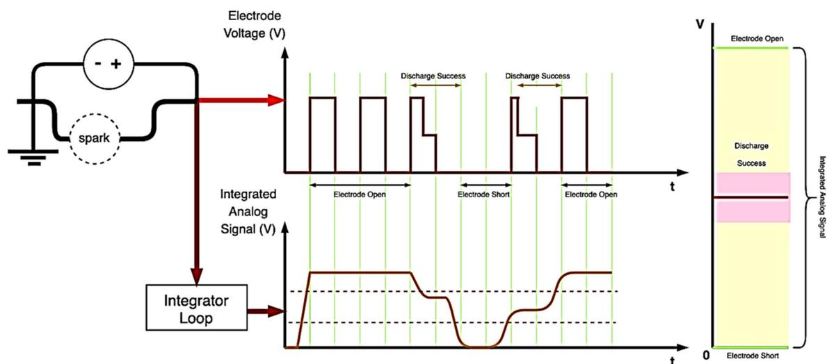
Figure 5. Schematic of discharge voltage signal conversion.
