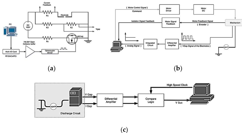
**Figure 3.** Circuit blocks of micro-EDM. (a) Discharge circuit, (b) motor control and signal feedback circuit, and (c) logic determination circuit.
