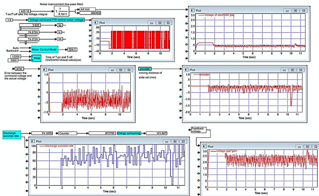
Figure 10. Process monitoring chart for preparing nano-bi.  $K_p = 3.622$ ,  $K_i = 74.2724$ , and  $K_d = 74.2724$ .
