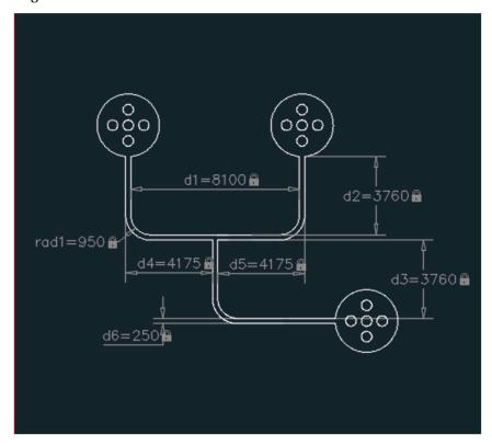
Figure S1. Mask drawing of silicon mold.
