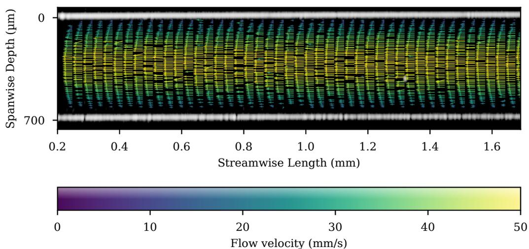
**Figure 7.** A flow velocity map is shown superimposed on a single OCT image frame from the straight section of the channel. The whole channel is shown with every third streamwise bin plotted for clarity. The bins are 10 μm square. The length of the velocity vector is additionally indicated by the colour bar. Missing arrows represent empty bins.
