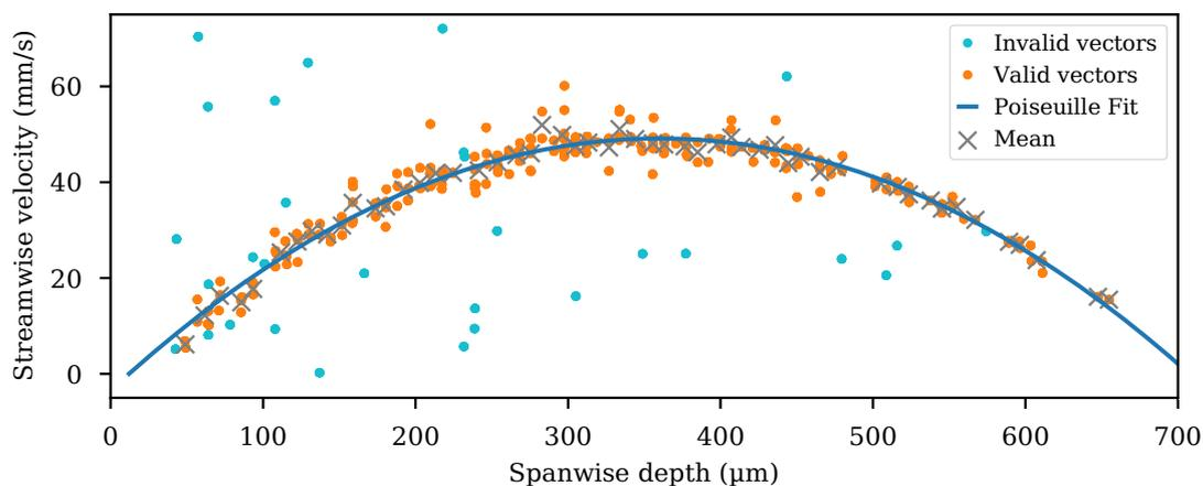
**Figure 5.** Valid and invalid flow velocity vectors shown spanwise across the microfluidic channel, for a single streamwise bin. The mean value of the valid vectors in each spanwise bin is shown. A parabolic Poiseuille fit to the valid vectors is shown. The top of the microfluidic channel as shown in Figure 2 appears at a  $0\ \mu\text{m}$  spanwise depth.
