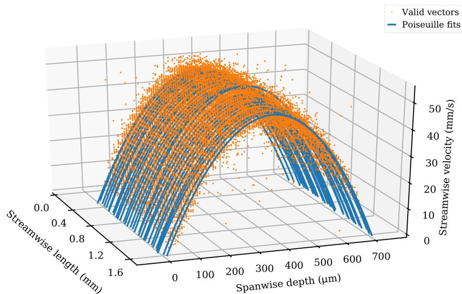
**Figure 6.** Spatially-resolved flow vectors and velocities for the straight channel microfluidic chip. Flow velocity is shown on the z-axis. The x-axis is divided into spatial bins of 10 μm. The y-axis is continuous. Orange dots represent individual valid velocity vectors, whilst blue lines represent the parabolic Poiseuille equation fits. There are 140,000 valid vectors. Only every second streamwise bin is plotted for clarity.
