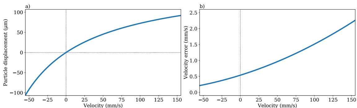
**Figure 4.** (a) Particle displacement between the image frames plotted against the particle velocity. (b) Velocity error per bin plotted against the particle velocity, assuming a half-pixel particle position error and 100 particles in each bin.
