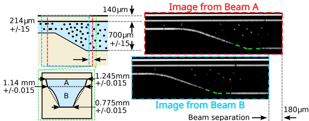
**Figure 3.** Schematic of the sloped section of the microfluidic chip with the area imaged by Beams A and B of the dual beam OCT instrument marked with blue and red outlines. The actual OCT images are shown with matching outline colours. The superimposed green dashed line marks the location of the slope. The spanwise width cross-section of the microfluidic channel is shown in the lower left outlined in green, including the PMMA slumping around the base of the channel.
