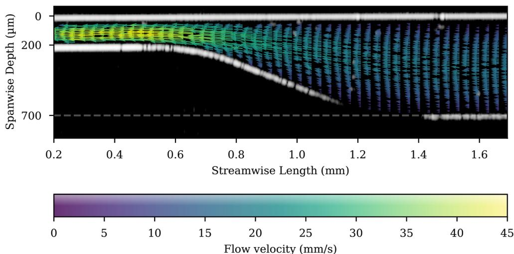
**Figure 8.** A flow velocity map is shown superimposed on a single OCT image frame from the sloped section of the channel. The whole channel is shown with every third streamwise bin plotted for clarity. The bins are 10  $\mu\text{m}$  square. The length of the velocity vector is additionally indicated by the colour bar. Missing arrows represent empty bins. The grey line at 700  $\mu\text{m}$  depth has been added to mark the position of the bottom of the channel on the x-axis.
