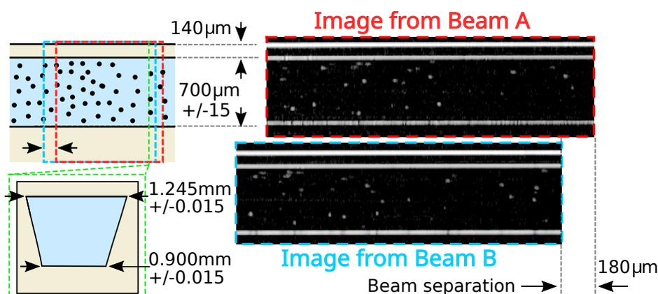
**Figure 2.** Schematic of the straight channel section of the microfluidic chip with the area imaged by Beams A and B of the dual beam OCT instrument marked and images from the dual beam OCT instrument with the appropriate beam separation. A cross-section of the microfluidic channel is shown in the lower left.
