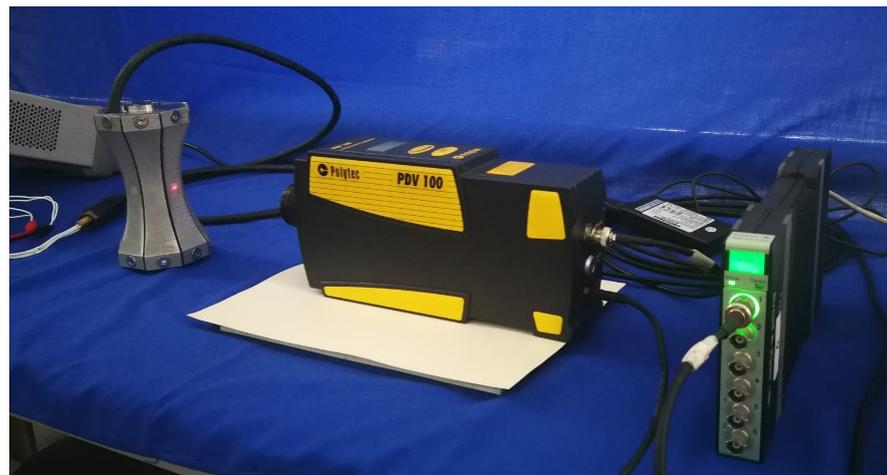
Figure 11. Implementation of vibration test using optical measurement equipment PDV 100 (in air).
