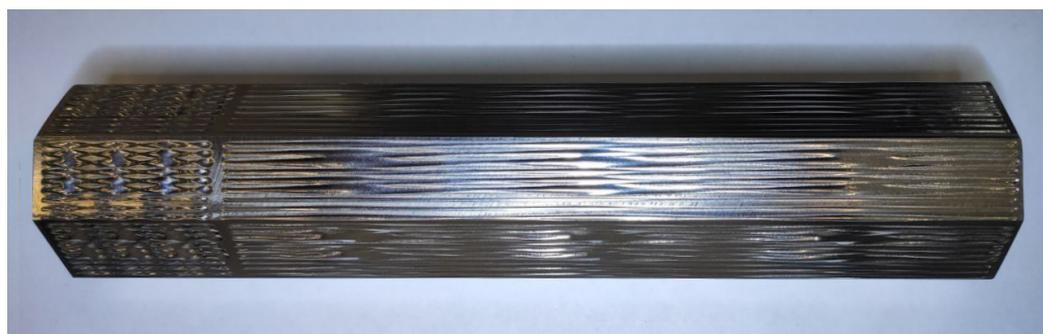
**Figure 4.** Octagonal Ti-6Al-4V alloy sample with textured single lines on the surface.
