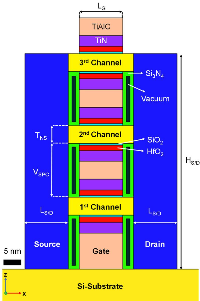
Figure 1. Cross-sectional schematic of an NS FET with vacuum inner spacer for ETA simulations.
