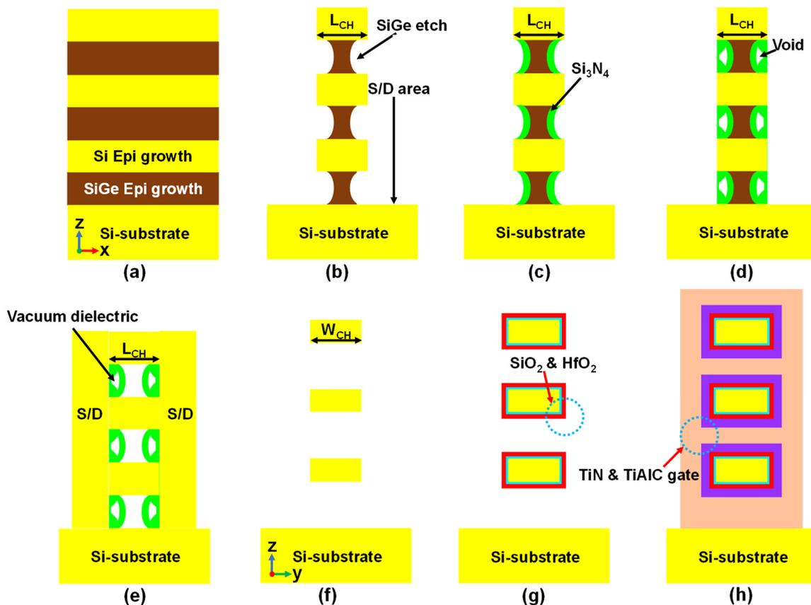
Figure 6. Proposed fabrication process flow of an NS FET with vacuum inner spacer. (a) Si/Si<sub>x</sub>Ge<sub>1-x</sub> epitaxial growths on Si substrate. (b) Si<sub>x</sub>Ge<sub>1-x</sub> indent etching. (c,d) Inner spacer deposition with void formation. (e,f) S/D epitaxial growth and suspended multiple nanosheet formation. (g,h) Gate dielectric and metal gate deposition.
