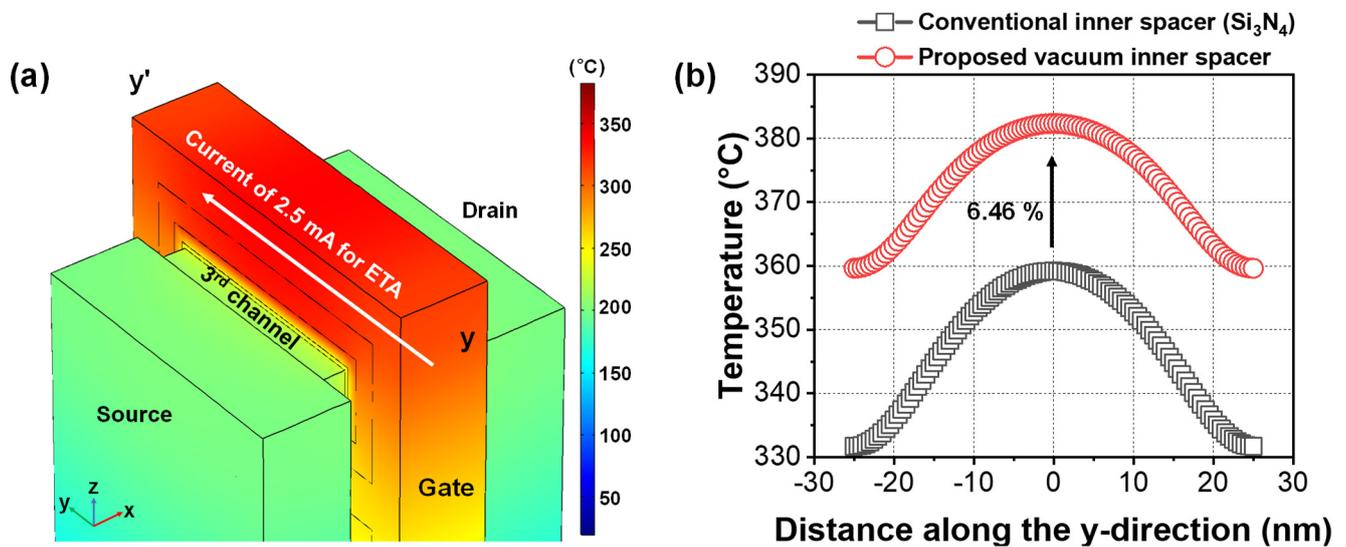
**Figure 2.** (a) Simulated heat distribution profile during ETA using gate-to-gate current in an NS FET. (b) Extracted temperature on the gate surface according to inner spacer material.
