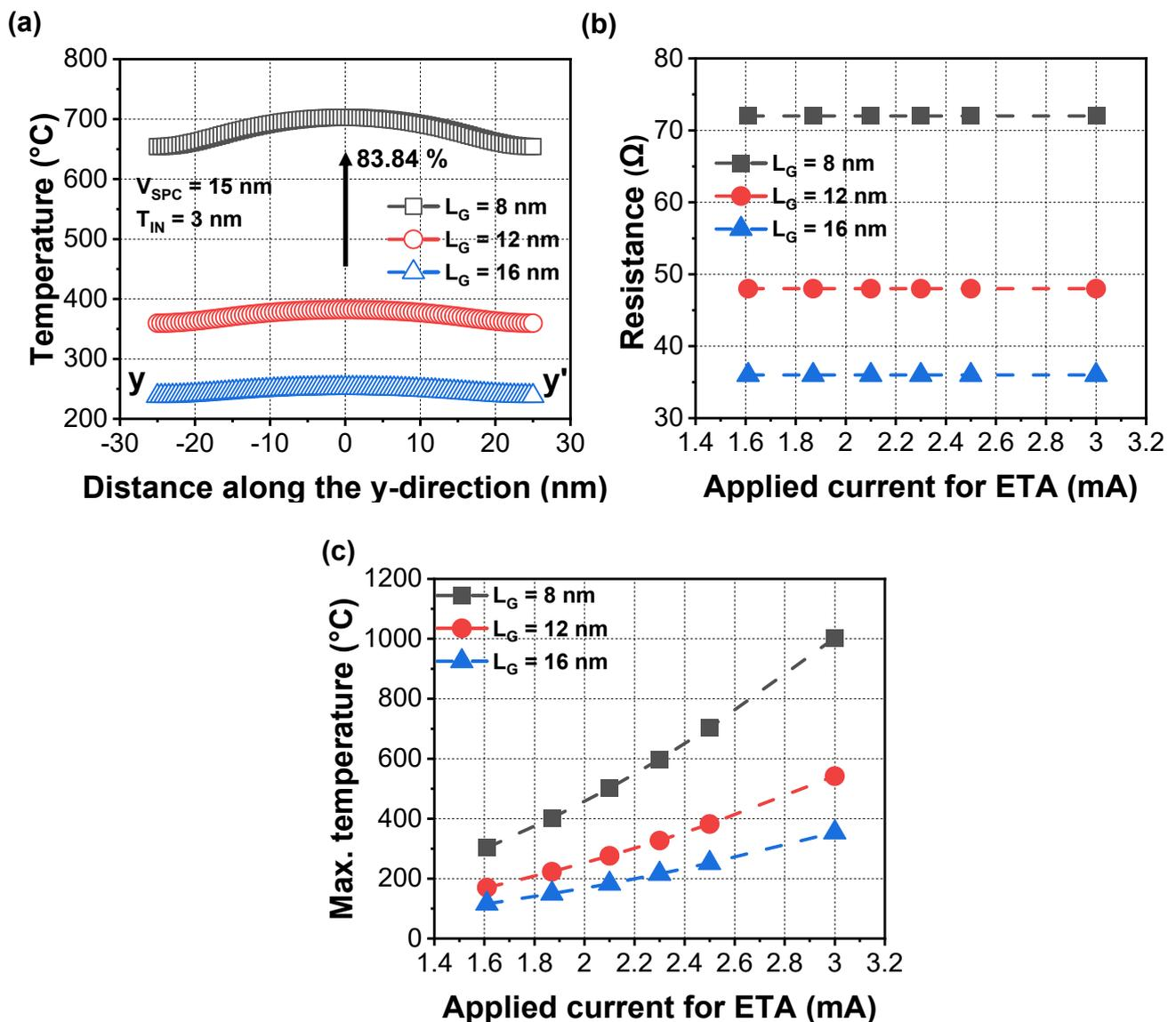
**Figure 3.** (a) Extracted temperature during the ETA in an NS FET with vacuum dielectric with respect to  $L_G$ . Extracted (b) gate to-gate resistance and (c) maximum temperature with various applied currents for the ETA, respectively. Inner spacer thickness ( $T_{IN}$ ) was fixed to 3 nm regardless of  $L_G$ .
