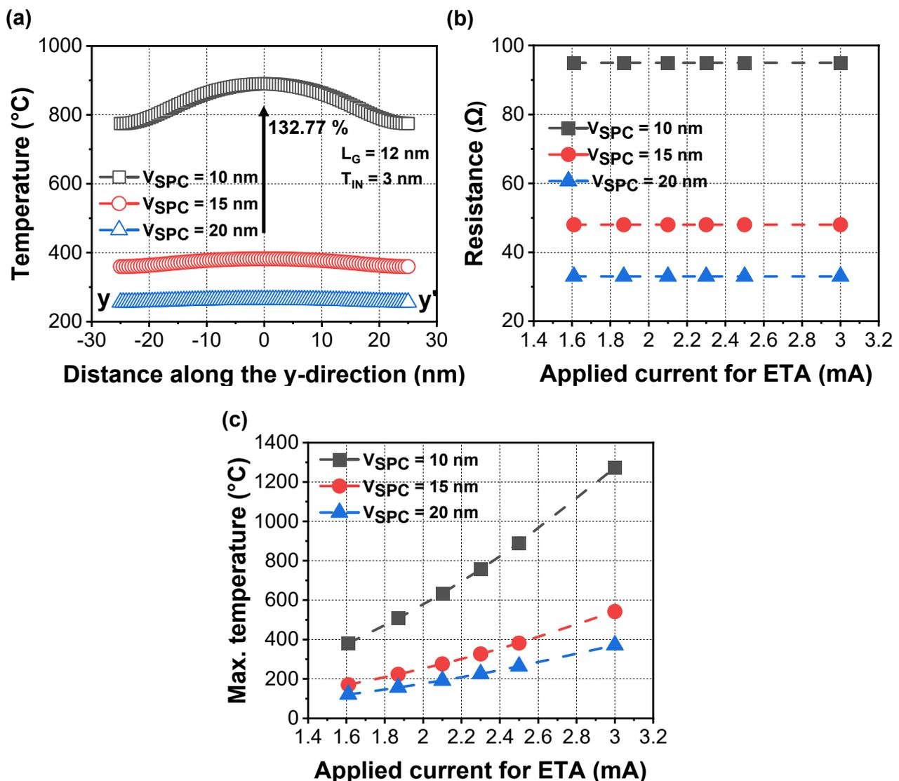
**Figure 4.** (a) Extracted temperature during the ETA in an NS FET with vacuum dielectric with various V<sub>SPC</sub>. Extracted (b) gate-to-gate resistance and (c) surface temperature with respect to V<sub>SPC</sub> and applied current, respectively.
