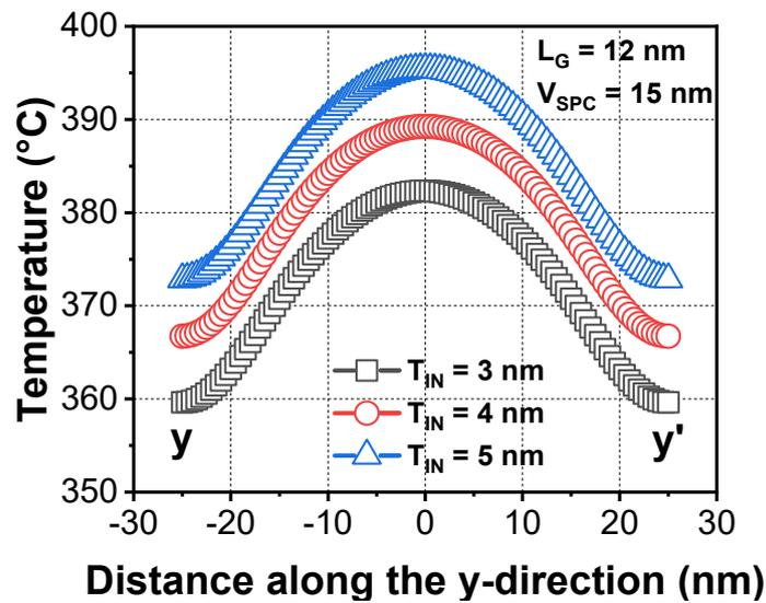
Figure 5. Extracted temperature during the ETA with various inner spacer thickness ( $T_{IN}$ ).
