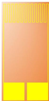
Figure 6. Structure diagram of resistance micro-temperature sensor.
