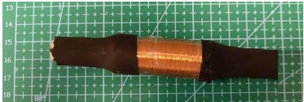
**Figure 5.** A finished microgenerator.
