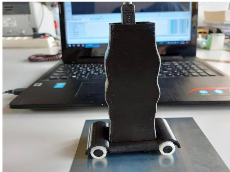
**Figure 14.** The final device in its 3D-printed packaging, connected to a laptop via a USB cable.
