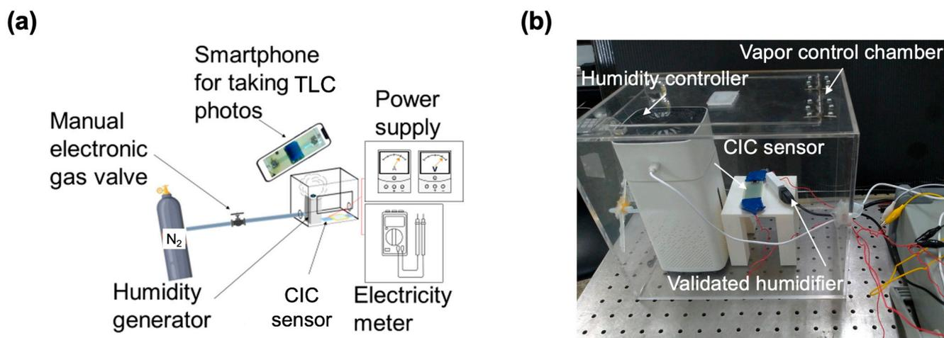
**Figure 2.** Experimental setup for CIC sensor evaluation. (a) Schematic illustrating the observation chamber designed for real-time measurements of ambient humidity. (b) Photograph providing an overview of the complete experimental setup. A commercial humidifier is employed to validate the readout obtained from the CIC sensor.
