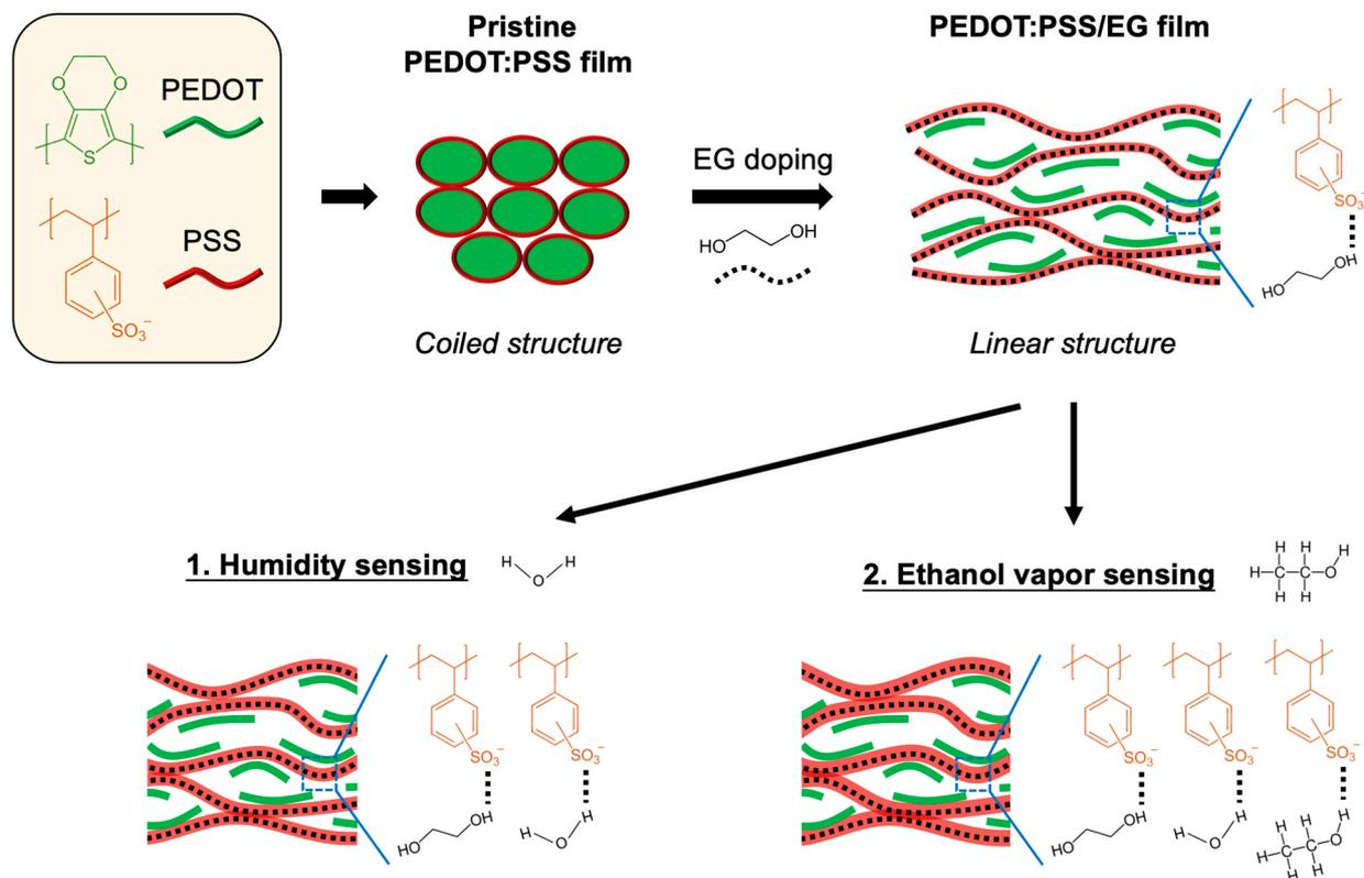
**Figure 7.** Schematic illustration of PEDOT:PSS with secondary EG doping for sensing both humidity and ethanol vapor.
