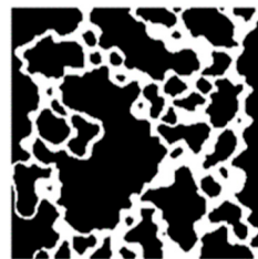
Figure 6. HO49Y. Hostun sand is relatively homogeneous, characterized by well-sorted predominantly quartz angular grains.
