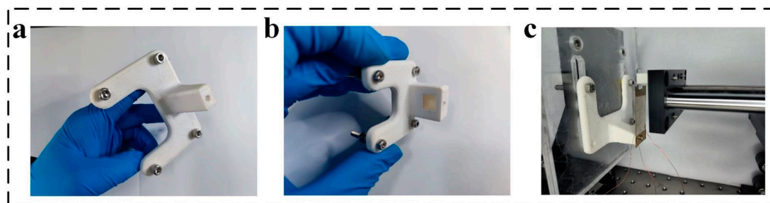
Figure S1. Physical structure of installation platform: (a) stator, (b) rotor, (c) assembly drawing.
