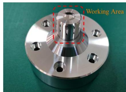
**Figure 8.** Standard workpiece.
