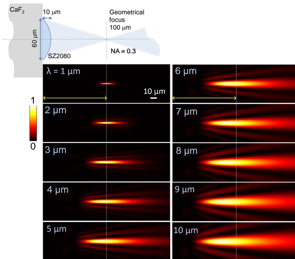
**Figure A2.** The Rayleigh–Sommerfeld (RS) diffraction integral, Equation (1). Calculation of the axial linearity distribution (normalised) at different wavelengths  $\lambda$  for the fixed refractive index  $n_{SZ2080} = 1.504$ . Simulations for the visible 633 nm wavelength using the same approach is shown in Figure 4.
