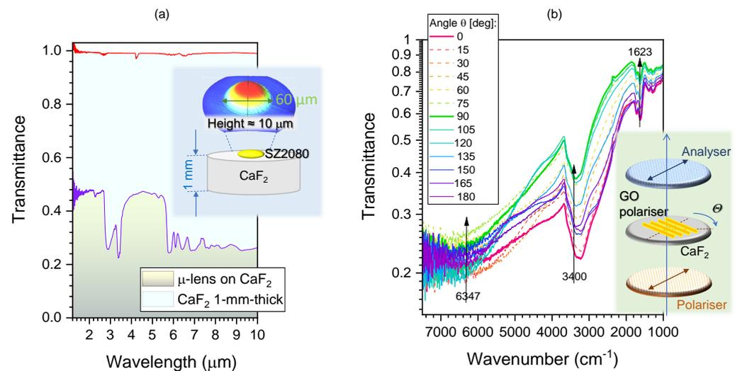
**Figure 6.** (a) IR transmittance spectra of the fabricated GO polariser measured by a microscope FTIR spectrometer with a parallel polariser–analyser. (b) Transmittance and the fitted formulae of the contributions from absorbance and the retardants at 1.58, 2.94, and 6.16  $\mu\text{m}$ , as marked in the transmittance spectra. Note that  $T$  is plotted on a logarithmic scale to better reveal any small changes. At 3530 and 1080  $\text{cm}^{-1}$ , C-OH vibrations are present [53].
