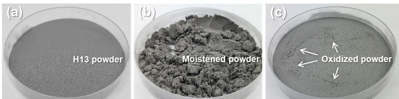
**Figure 5.** Images of (a) the original H13 powders and (b,c) the oxidized H13 powders at 70 °C for 72 h. The image (c) shows the oxidized powders after being dried.
