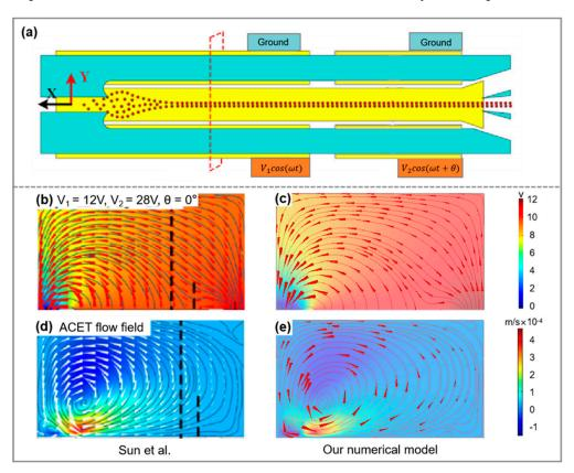
**Figure 2.** (a) The schematic of the separator proposed by Sun et al. [25], with the section containing the simulation results highlighted by the dashed line; (**b**,**c**) represent the electric field distributions calculated from Sun et al. and in this work, respectively; and (**d**,**e**) depict the flow field distributions calculated from Sun et al. and in this work, respectively. ( $u = 25 \times 10^{-6} \text{ m/s}$ ,  $\sigma_m = 0.1 \text{ S/m}$ , and f = 1 MHz).
