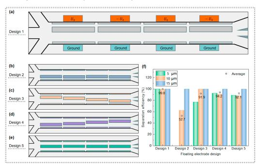
Figure 5. The arrangement of floating electrodes and its influence on particle separation efficiency: (a–e) different floating electrode arrangements and (f) separation efficiency of PS particles with different floating electrode arrangements.
