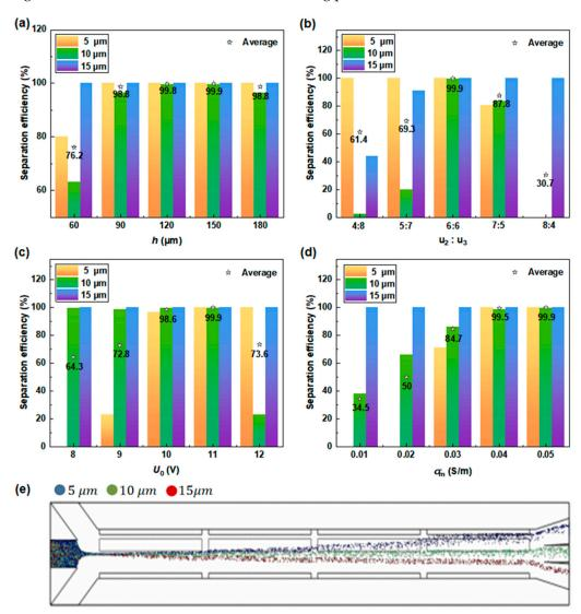
**Figure 6.** Study on single parameters affecting particle separation efficiency: separation efficiency of PS particles at (a) different particle inlet heights; (b) different sheath flow rates; (c) different driving voltages; (d) different media conductivity; and (e) particle trajectories with sizes of 5, 10, and 15  $\mu$ m under the optimal operating parameters.
