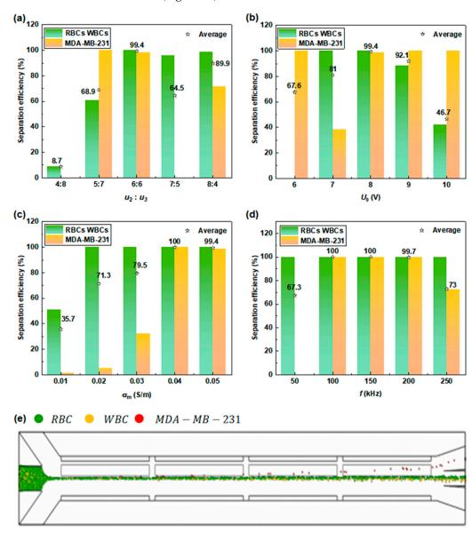
**Figure 7.** Study on operating parameters affecting the separation efficiency between normal blood cells and CTCs: (a) sheath flow rates; (b) driving voltages; (c) medium conductivities; and (d) electric field frequencies. (e) Trajectories of cells under the following optimal operating parameters:  $u_1 = 3 \times 10^{-4}$  m/s,  $u_2 = u_3 = 6 \times 10^{-4}$  m/s,  $u_3 = 8$  V,  $u_4 = 0.04$  S/m, and  $u_4 = 0.04$  S/m, and  $u_4 = 0.04$  kHz.
