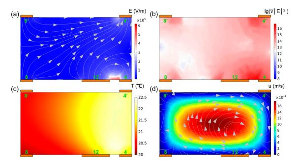
**Figure 4.** Physical field distribution diagram of the separator cross section at  $x = 2900 \mu m$ : (a) electric field strength; (b) the gradient of electric field strength squared; (c) temperature field; and (d) fluid flow velocity.
