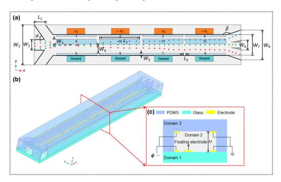
**Figure 1.** Design layout of the (bio)microparticle separator: (a) top view of the separator and illustration of particle separation trajectories; (b) 3D geometric model of the separator; and (c) cross-section view of the separator.
