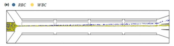
**Figure 8.** Study on single parameters affecting the separation efficiency of RBCs and WBCs. Separation efficiency of RBCs and WBCs at different (a) sheath flow rates, (b) driving voltages, (c) media conductivity, and (d) frequencies. (e) The trajectories of RBCs and WBCs under optimal operating parameters.
