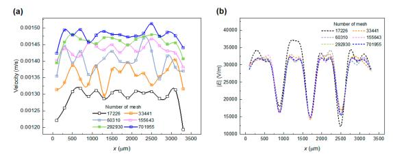
Figure 3. Mesh-independence analysis: (a) flow velocity curves and (b) electric field strength curves.
