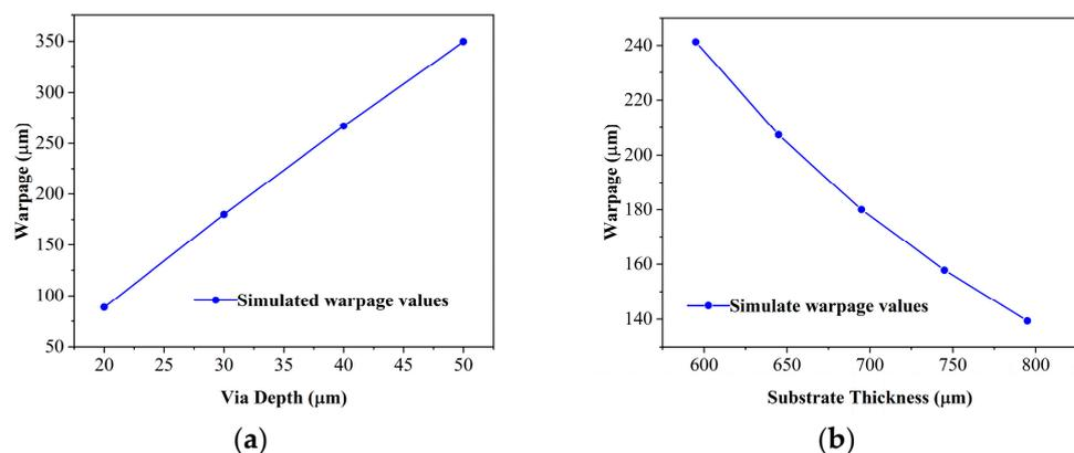
Figure 9. The effect of (a) via depth, (b) substrate thickness on wafer warpage.
