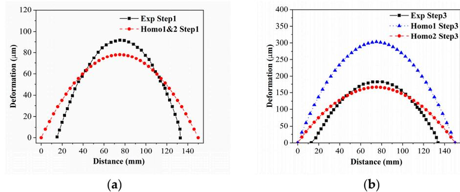
**Figure 7.** Experimental measurement of wafer warpage compared with two homogenization results (Exp: experiment results, homo 1: direct homogenization results, homo 2: multi-step homogenization results). (a) After process step 1: SiO<sub>2</sub> layer deposition; (b) After process step 3: Poly-Si layer deposition.
