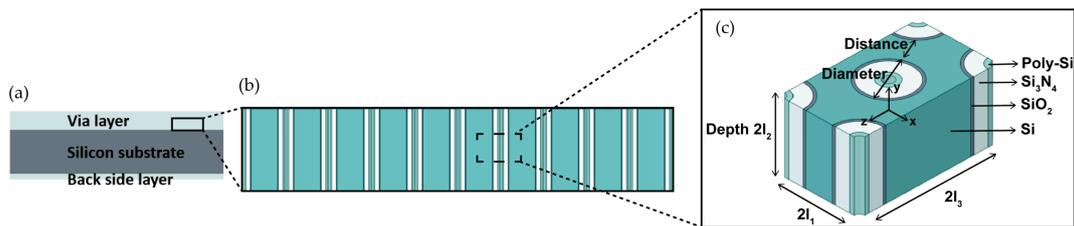
**Figure 2.** The extraction process and the dimensions of the RVE. (a) Side view of the wafer; (b) Side view of the via layer; (c) Representation of the RVE structure.
