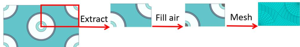
**Figure 3.** A top view illustration showcasing the RVE model and its homogenization process.
