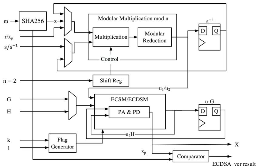
Figure 4. The hardware architecture of ECDSA.
