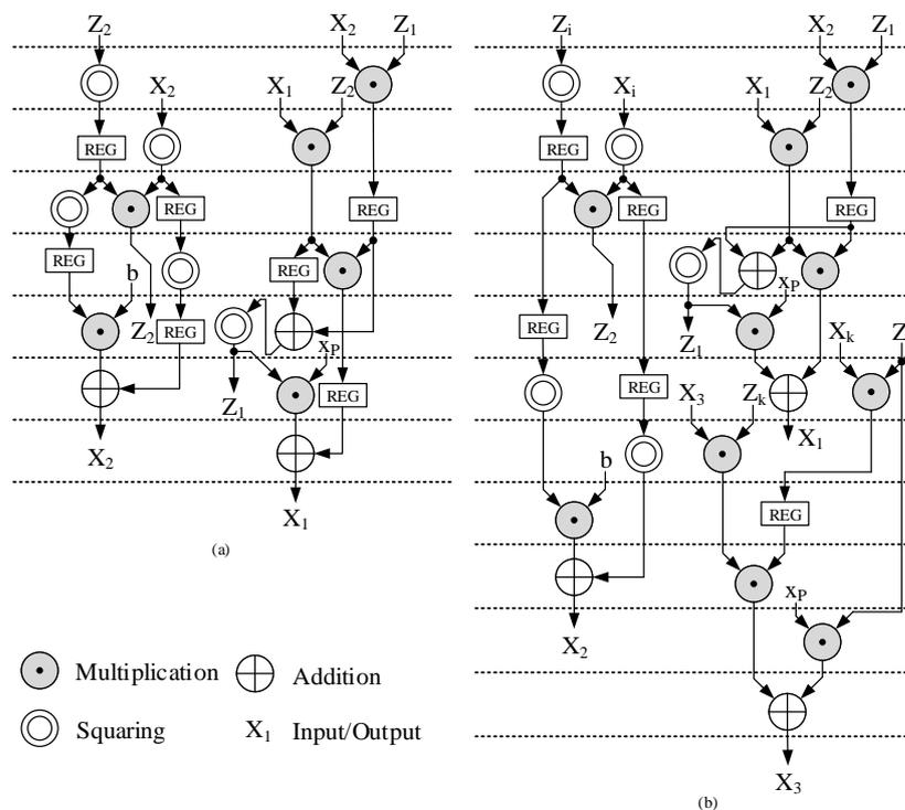
Figure 5. The proposed timing schedule of (a) ECSM and (b) ECDSM.
