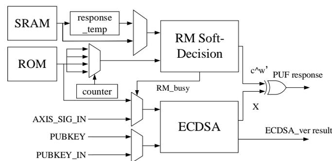
**Figure 1.** The overall structure of ECDSA-PUF.
