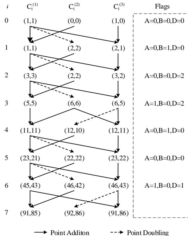
**Figure A2.** An example of ECDSM ( $91P + 85Q$ ) with a two-dimensional DAC.
