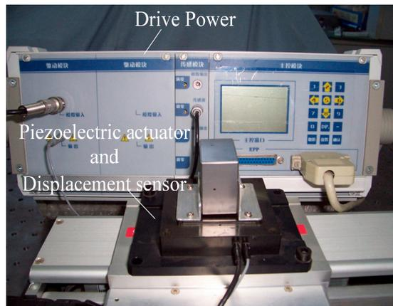
Figure 3. The PZA experiment devices.
