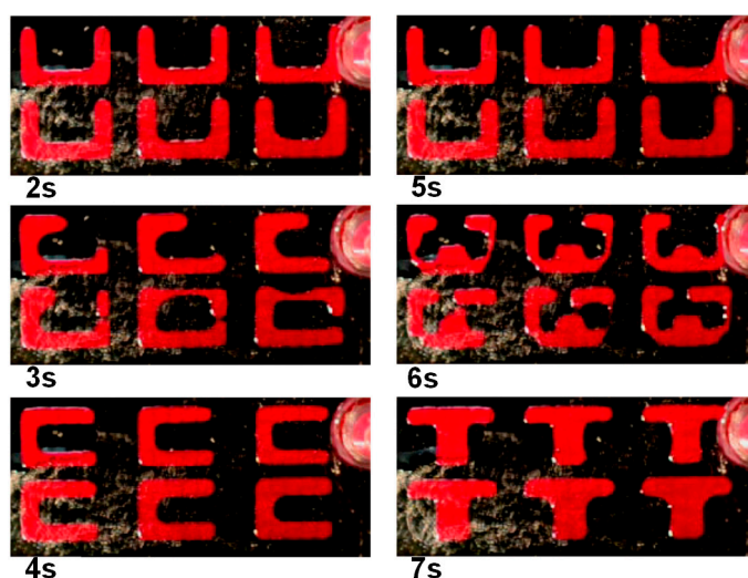
Figure 5. A six-unit array was supplied with red fluid in portioned volumes, and the user interface was programmed to transition between the patterns every two seconds. Panels show the transition from U to C and U to T. Refer to ESI3 for the video.
