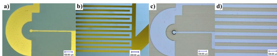
**Figure 1.** Platinum (a,b) and indium tin oxide (ITO) (c,d) structures of the oxygen sensors with a circular working electrode spot and semi-circular counter electrodes (a,c), as well as interdigitated electrode structures (IDES) with a 50- $\mu\text{m}$  pitch (b,d). The on-chip-sensor connectors were insulated in a following processing step.
