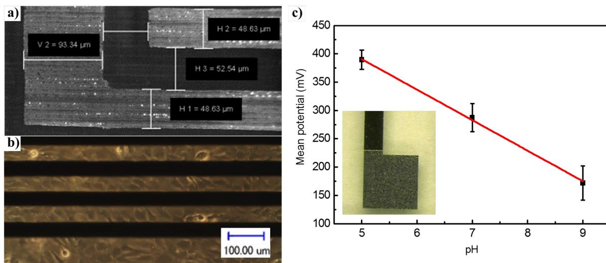
**Figure 4.** Images of a platinum IDES. (a) Scanning electron microscopy image with dimensions. (b) Confluent cells above the IDES. (c) Sensitivity test of a Si<sub>3</sub>N<sub>4</sub> sensor layer on platinum (insert: pH sensor with 1.4 × 1.4 mm<sup>2</sup> electrode area). The data represent measurements with six chips in pH-buffered solutions with pH values of 5, 7, and 9. The straight line corresponds to a sensitivity of  $-53.8 \pm 1.8$  mV/pH.
