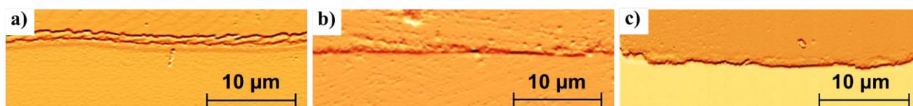
**Figure 3.** Edge quality of an IDES finger controlled by colour contrasted atomic force microscopic images. (a) ITO on glass; (b) platinum on glass; (c) photolithographically (photo mask) produced chip (GeSiM®).
