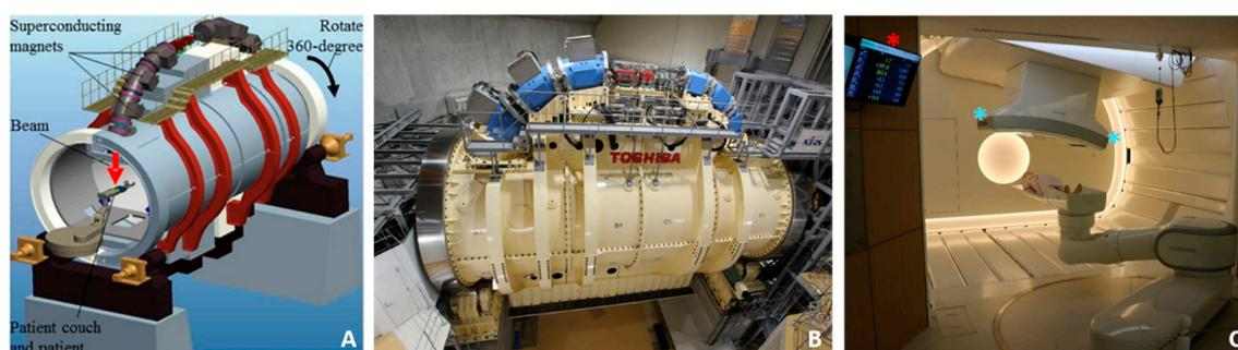
**Figure 4.** (A) Schematic diagram of the actual gantry seen in (B). Superconducting magnets, beam nozzle, and patient location are labelled. (C) A photograph showing a phantom patient on the robotic couch with the gantry in a slightly titled position. Also seen in the picture: the computer-based patient positioning system coordinates (red asterisk) and the flat panel detectors (blue asterisks).
