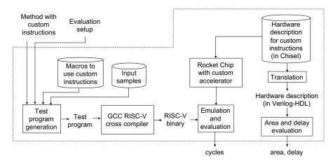
**Figure 10.** Overview of RISC-V-based evaluation environment. The dotted region is the framework proposed in Reference [21].
