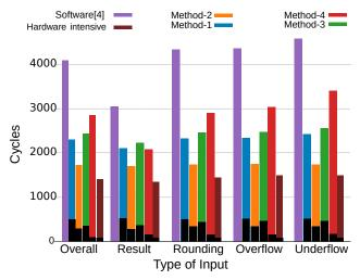
**Figure 13.** Comparison of the execution cycles for different input types. Each bar shows the average execution cycle for each pair of solution and input type. The black color indicates the cycles used by the hardware, e.g., the bar with blue and black colors shows the total execution time for Method-1, and the black area shows the cycles for the hardware.
