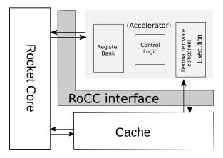
Figure 11. High-level architecture of Rocket Chip with Rocket Custom Coprocessor (RoCC) interface with accelerator.
