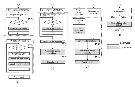
**Figure 6.** Flow of the proposed methods: (a) Method-1, (b) Method-2, (c) Method-3, and (d) Method-4. White and gray blocks indicate software parts and hardware parts, respectively.
