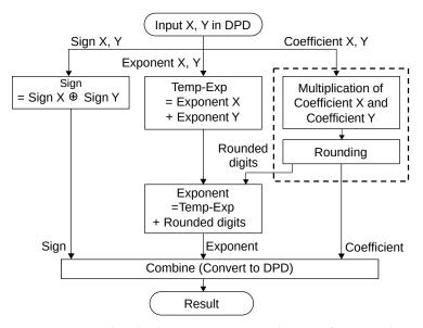
**Figure 2.** Decimal multiplication process. Hardware–software co-design solutions are considered in the dotted rectangle in this paper.
