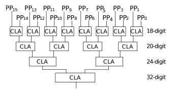
Figure 8. Parallel Accumulator for 64-bit operation.
