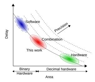
Figure 1. Area-delay relationship with precision for decimal arithmetic.
