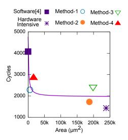
Figure 14. Area-delay tradeoff for the 64-bit precision.
