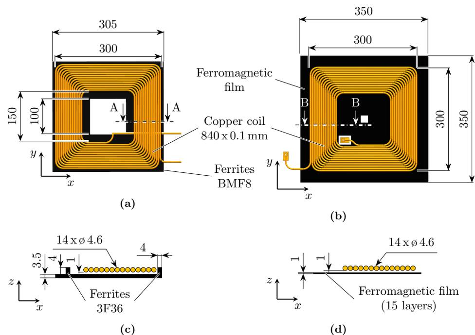
**Figure 7.** Dimensions of the CPM components (unit: mm): (a) sandwich concept and space-frame concept; (b) shell concept; (c) section A-A; (d) section B-B.
