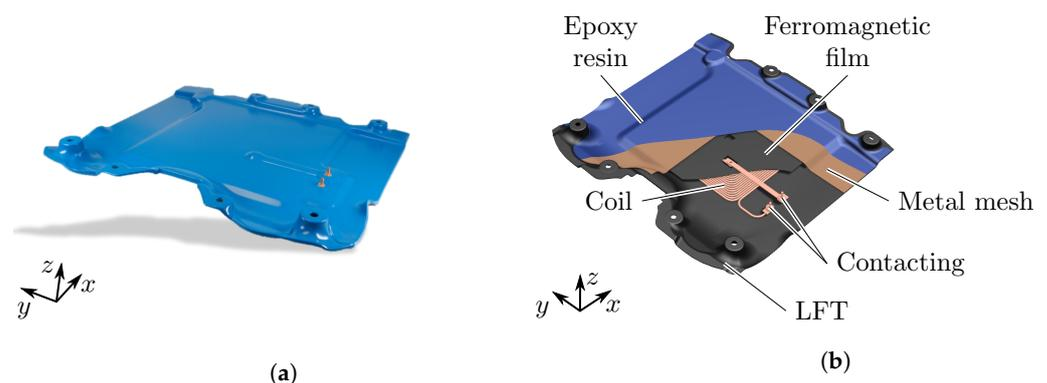
**Figure 8.** Generic prototype of the proposed shell concept: (a) photograph; and (b) exploded view.
