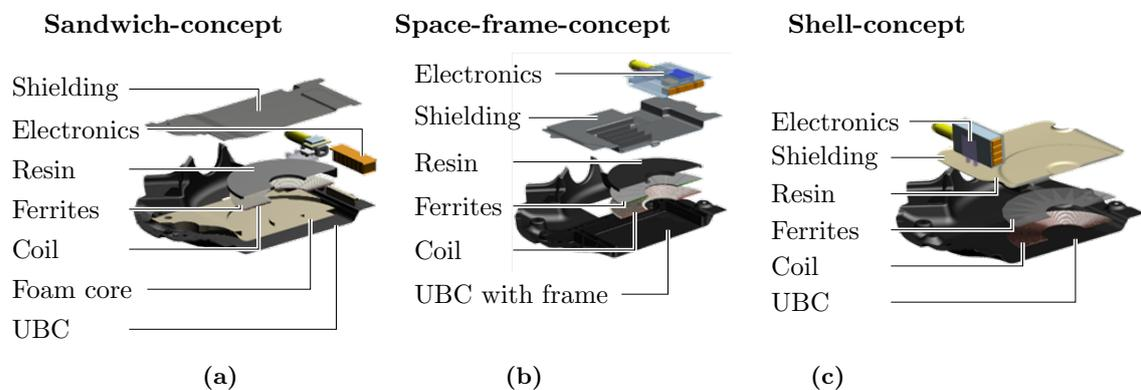
Figure 6. Proposed concepts of functionally integrated CPMs: (a) sandwich concept; (b) space-frame concept; and (c) shell concept.
