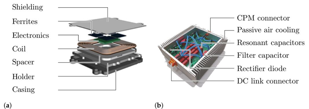
**Figure 3.** Components of conventional CPMs: (a) CPM; and (b) external power electronics.
