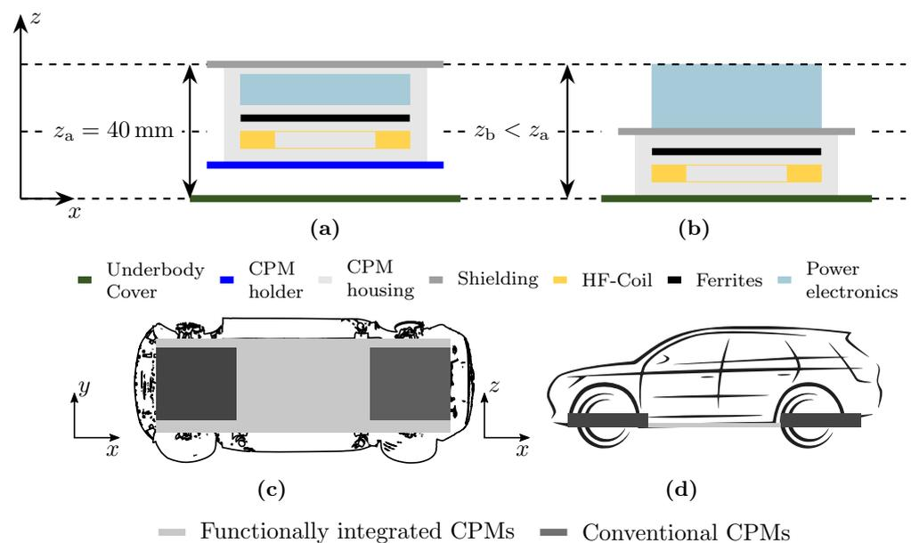
**Figure 4.** Qualitative comparison of the z-dimension of: (a) conventional designs of CPMs with a maximum transmission power of 3.6 kW given in [12]; (b) the functionally integrated CPM to be developed with a transmission power of more than 3.6 kW; and (c,d) possible installation space of CPM designs in (c) xy-plane and (d) xz-plane.
