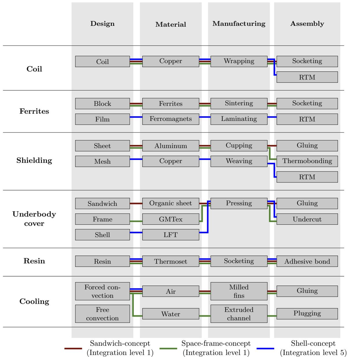
Figure 5. Proposed morphological box to the conception of functionally integrated CPMs.
