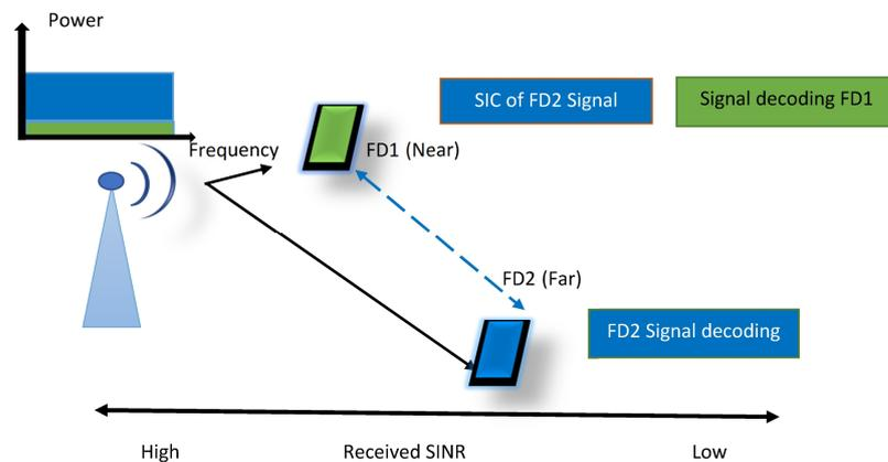
Figure 2. Decoding processes for the CR-NOMA system.
