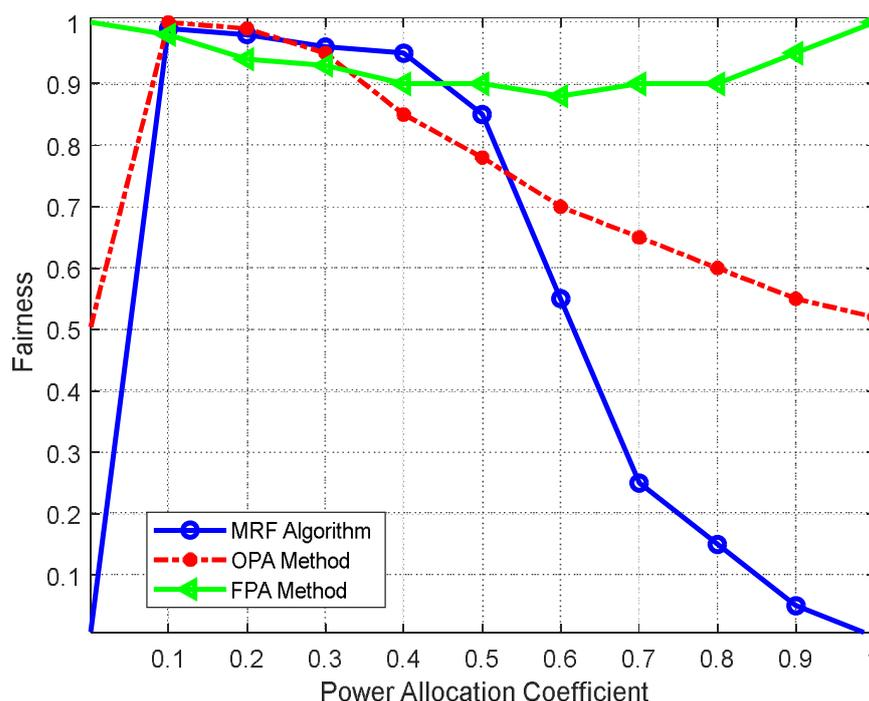
**Figure 5.** Fairness vs. coefficient power allocation with strong channel gain.
