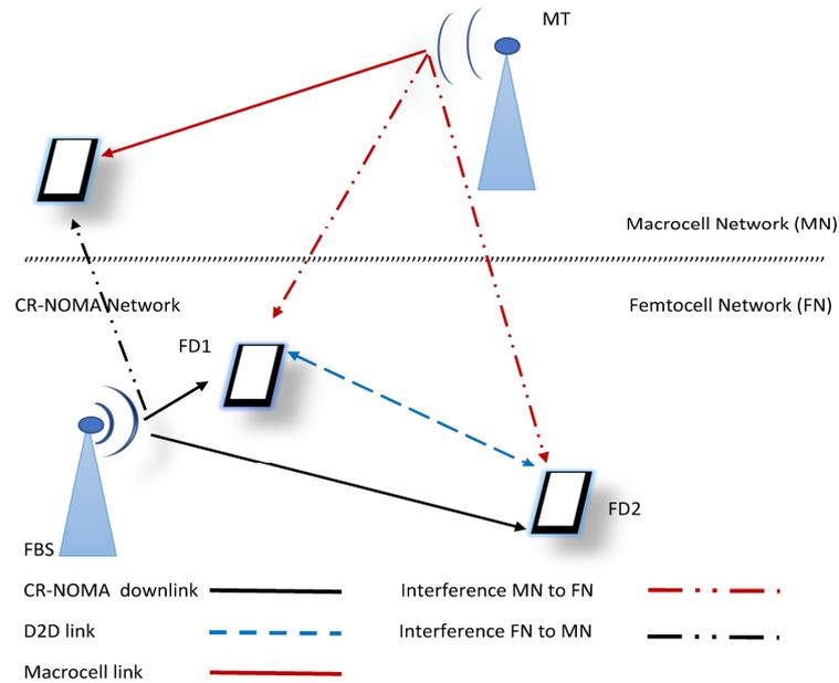
Figure 1. System model of CR-NOMA femtocell D2D link.
